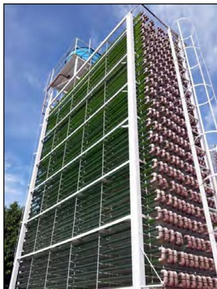
Figure 2. Tubular compact photobioreactor
