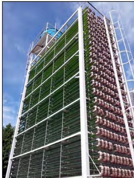
Figure 2. Tubular compact photobioreactor
