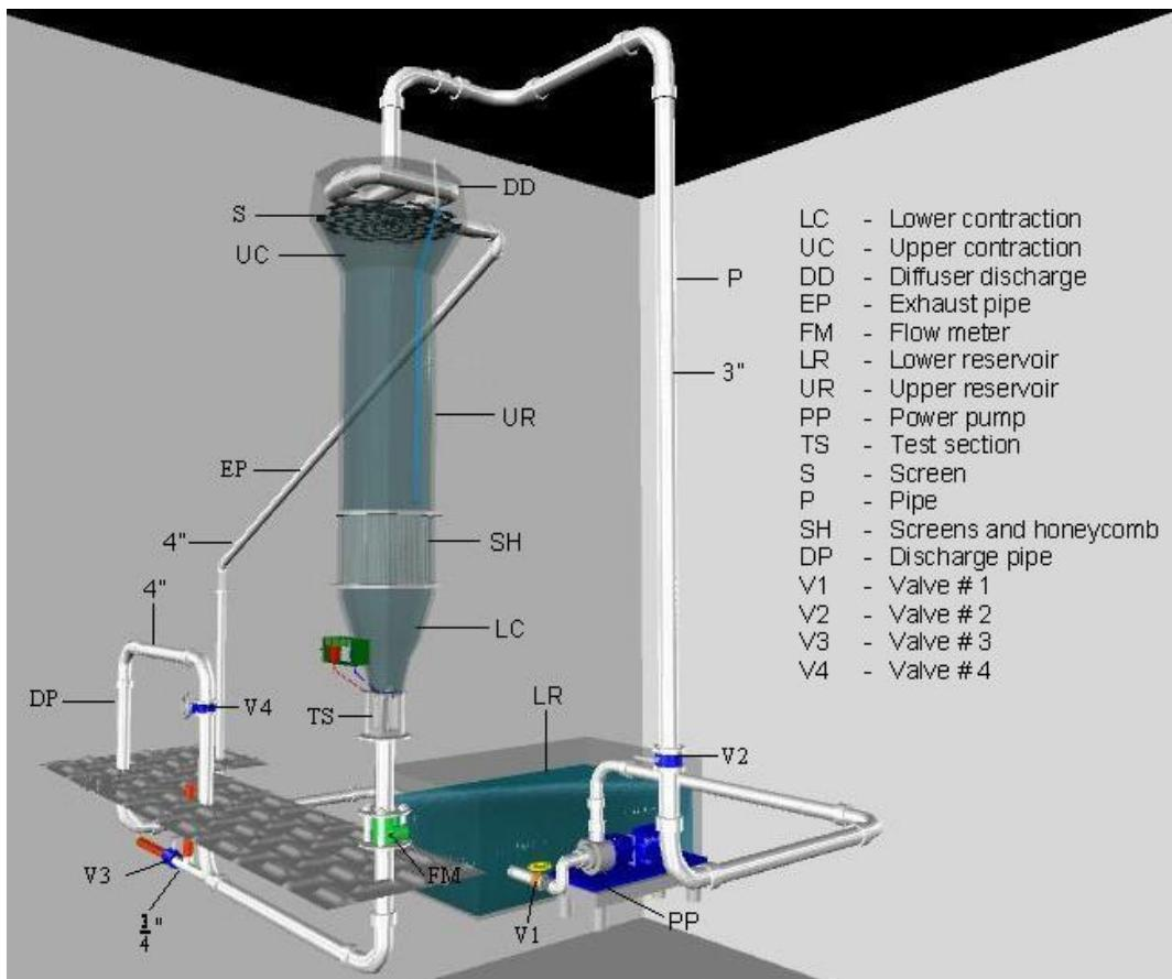
(a). The vertical hydrodynamic tunnel of the Flow Visualization Laboratory.
