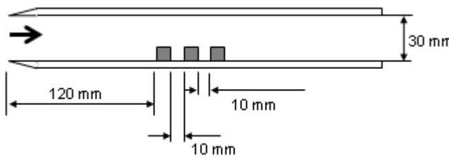
Figure 1. Channel with rectangular protuberances - geometry of the problem studied.
