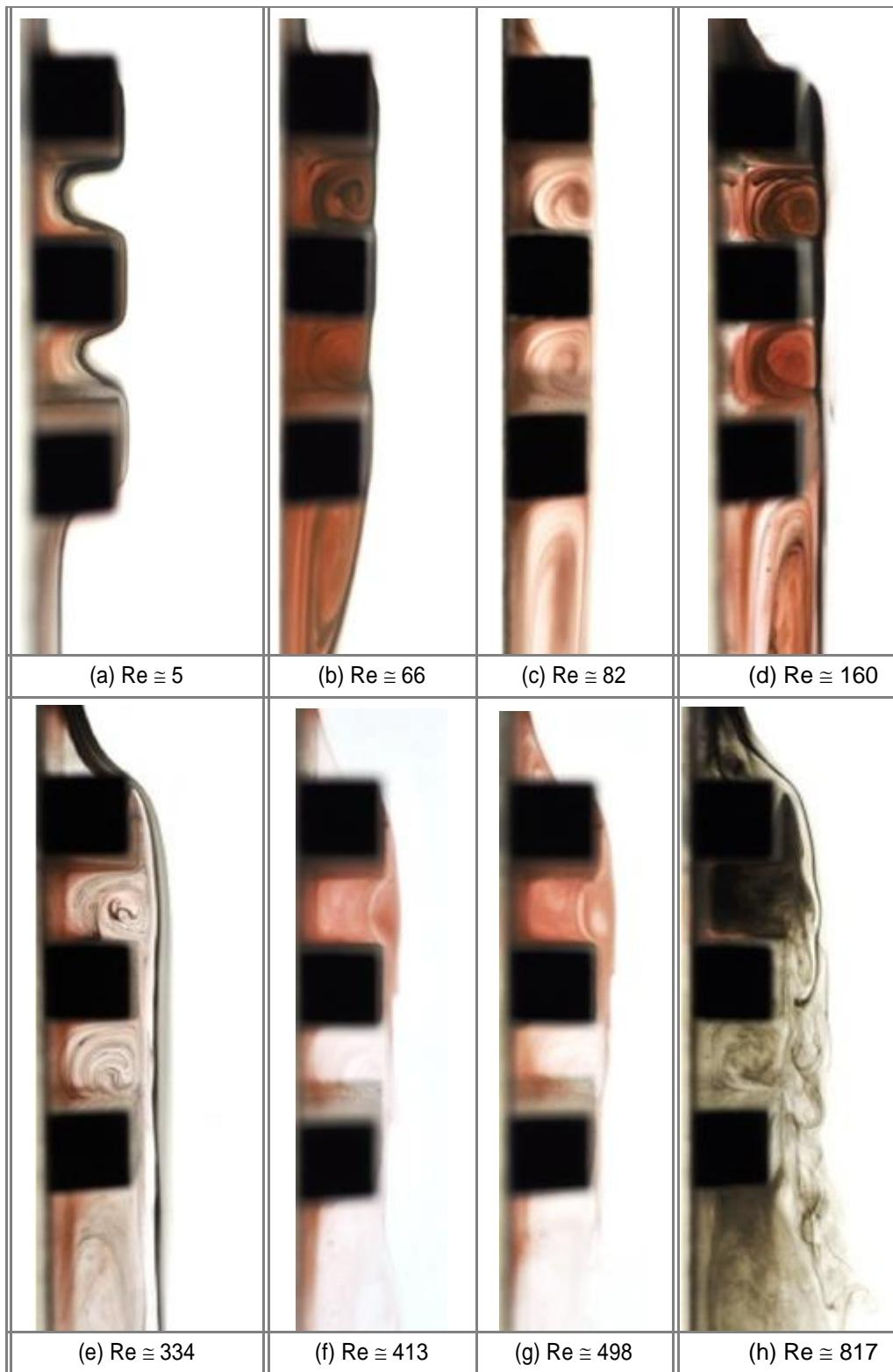
Figure 3. Experimental result for different number of Re.
