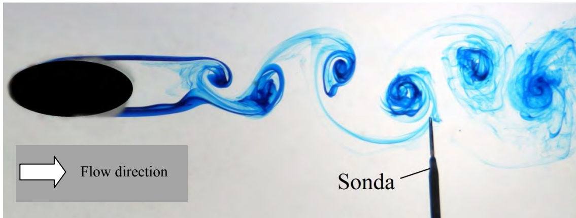
Figure 8. Hot film probes positioned in the wake of the elliptic cylinder.
