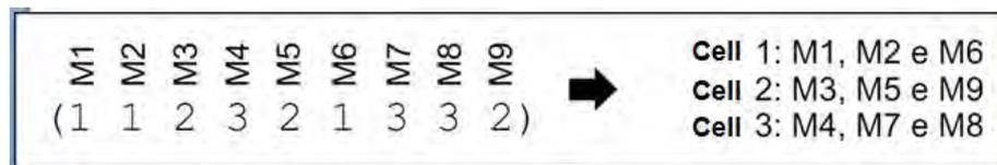
Figure 5. Representation of a chromosome for cell formation.
