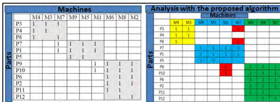
Figure 12. Comparison of the response obtained in the work analyzed and proposed application
