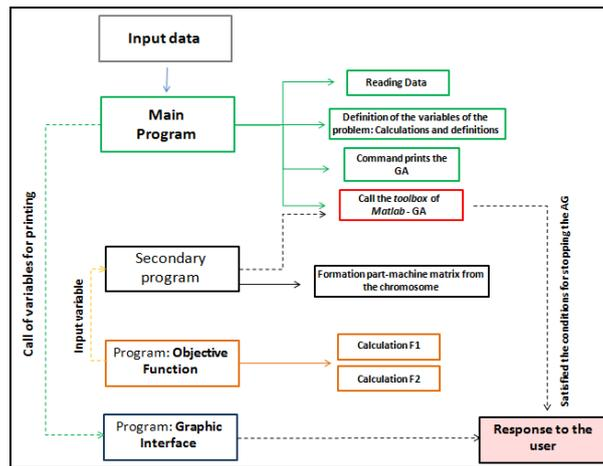
Figure 9. Principle of operation of the proposed algorithm
