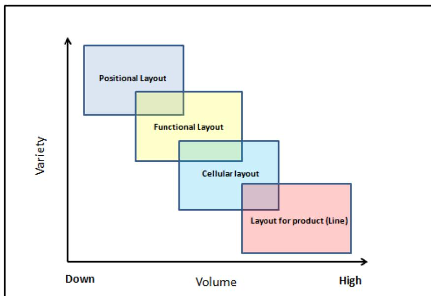
Figure 1. Relationship between variety–volume in the selection of a physic arrangement.
