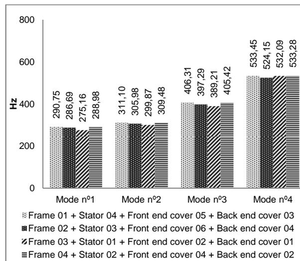
Figure 7 - Results of the natural frequencies of the frames with stators and the both end covers in the fixed condition.
