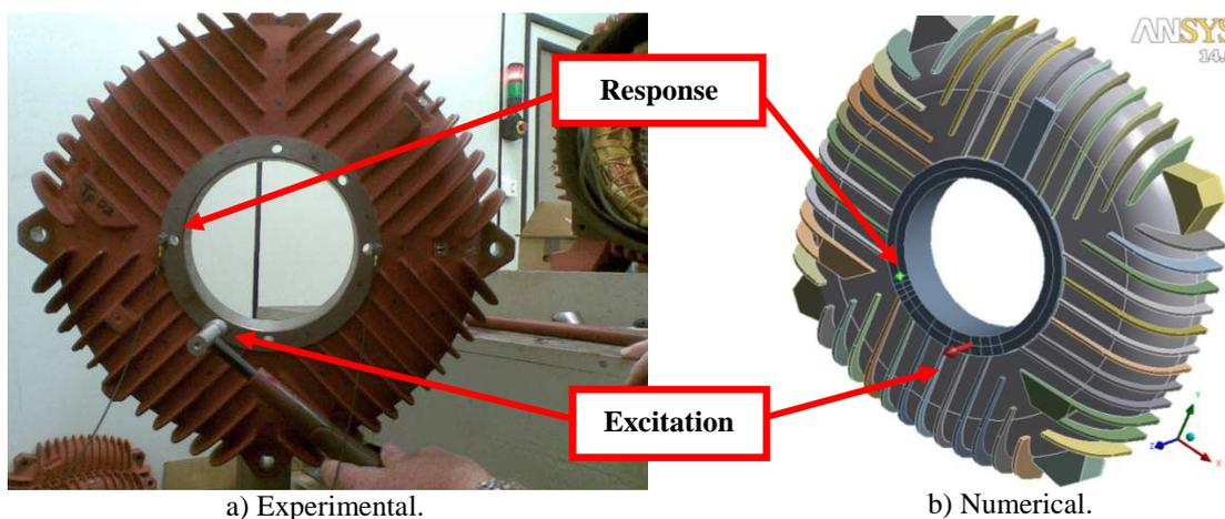
Figure 13 – Location example of the excitation and response points to obtain the FRF curves in the front end cover.
