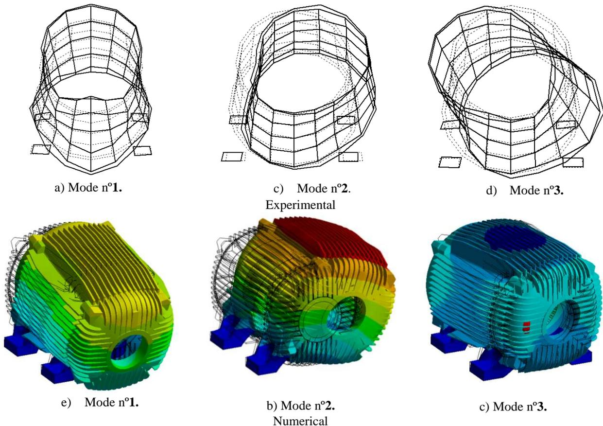
Figure 15 – First three experimental and numerical modes of vibration of the studied electric motor fixed on a rigid base.
