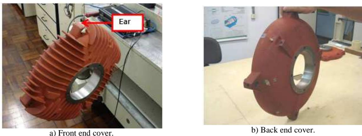
Figure 3 – Differences between front and back end covers.
