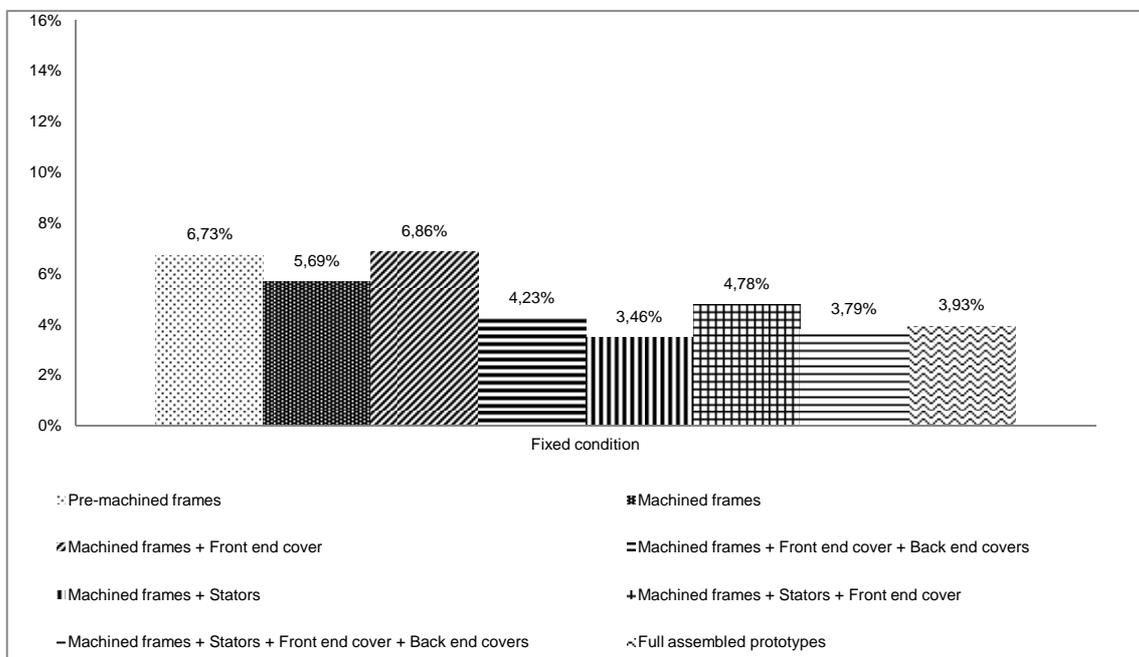
Figure 5 - Percentage variation of the experimental results of the first four natural frequencies of each component or set of components of the motor in fixed condition.
