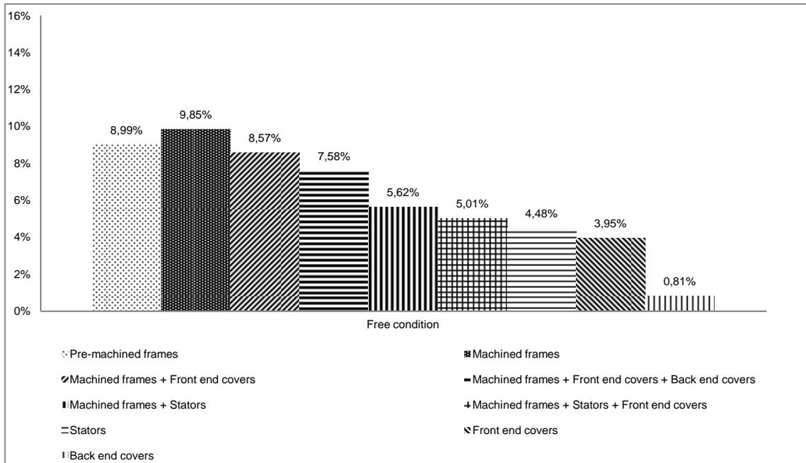
Figure 4 - Percentage variation of the experimental results of the first four natural frequencies of each component or set of components of the motor in free condition.
