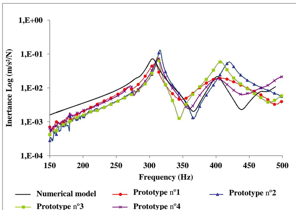
Figure 14 – Numerical and experimental FRF curves for the full prototypes mounted on a fixed base – Mean damping factor = 1,87%.
