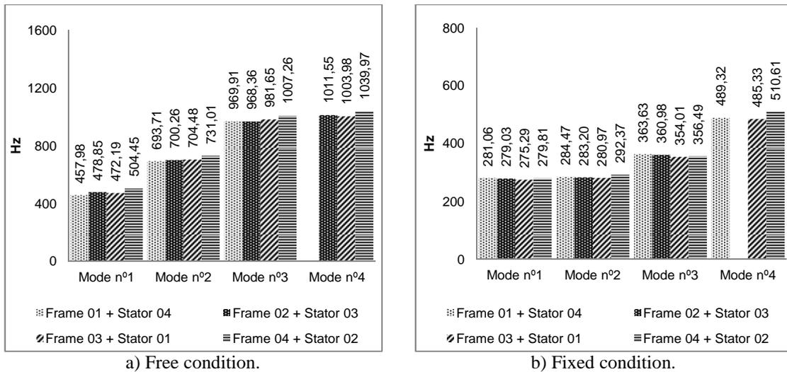
Figure 6 - Results of the natural frequencies of the frames with stators.
