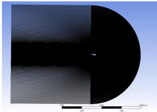
Figure 9. Refinement in the semicircle and, after the trailing edge, refinement until the end of the computational domain.
