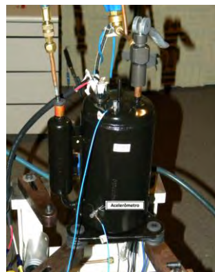
Figure 4. Position of accelerometer in welding point near the region of the accumulator.
