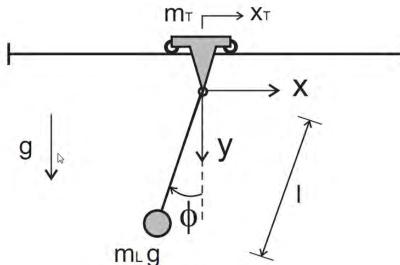
Figure 1 – Schematic of the Cart-pendulum System, Source: Puglia et al. (2011).
