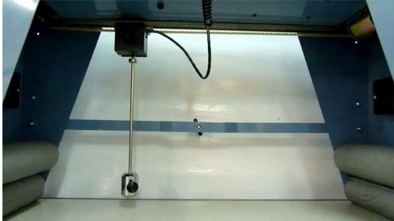
Figure 5. Byronic Cart-pendulum System.
