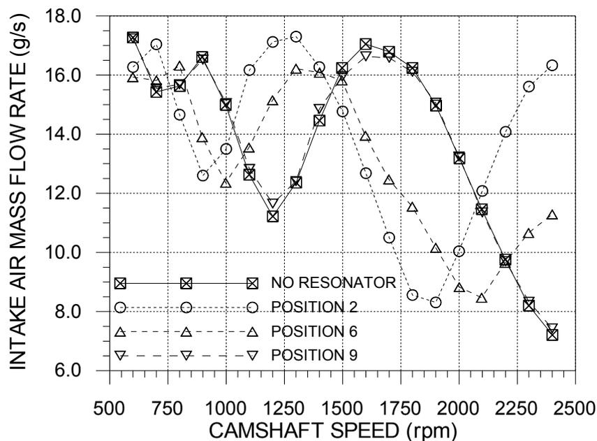
Figure 6 – Variation of intake air mass flow rate with camshaft speed for 114Hz Helmholtz resonator at three different positions.
