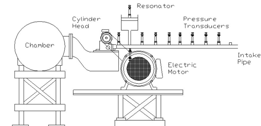
Figure 1 - Schematics of intake pipe with Helmholtz resonator.
