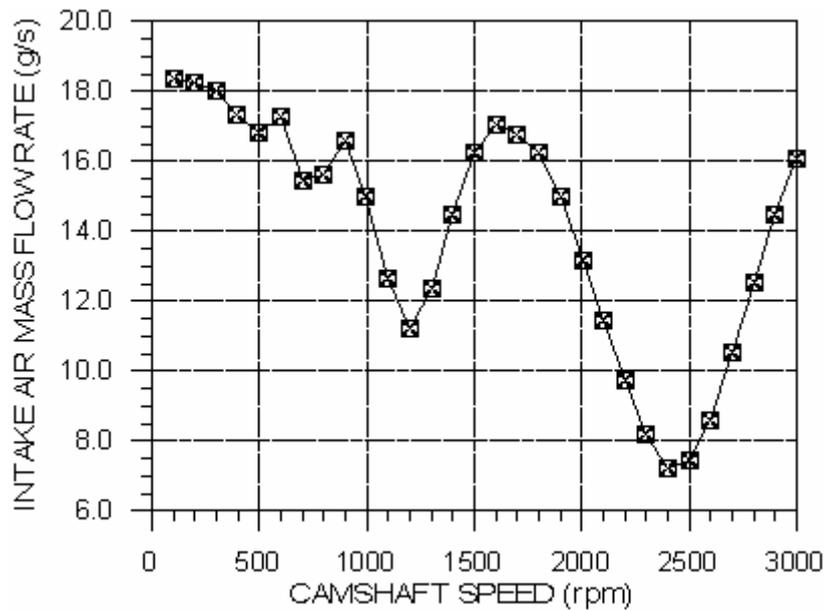
Figure 4 – Intake air mass flow rate for varying camshaft speed.
