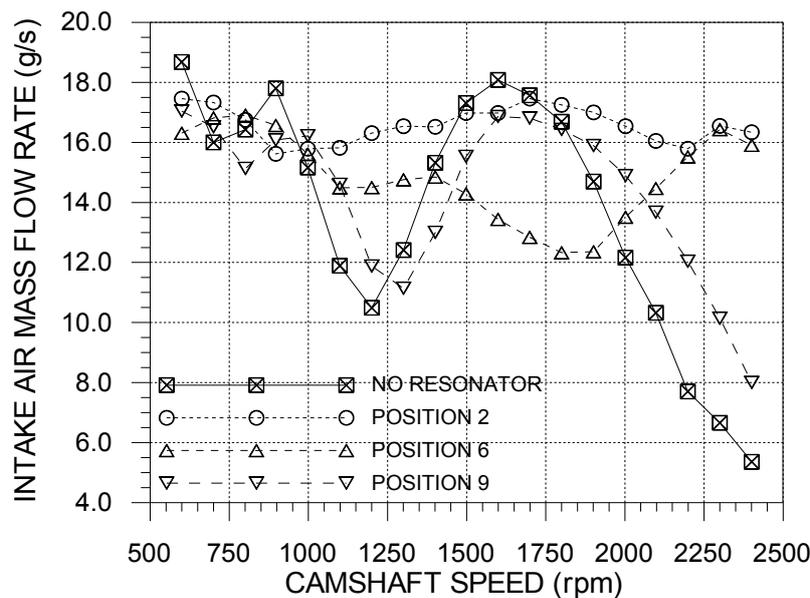
Figure 7 – Variation of intake air mass flow rate with camshaft speed for 40Hz Helmholtz resonator at three different positions.
