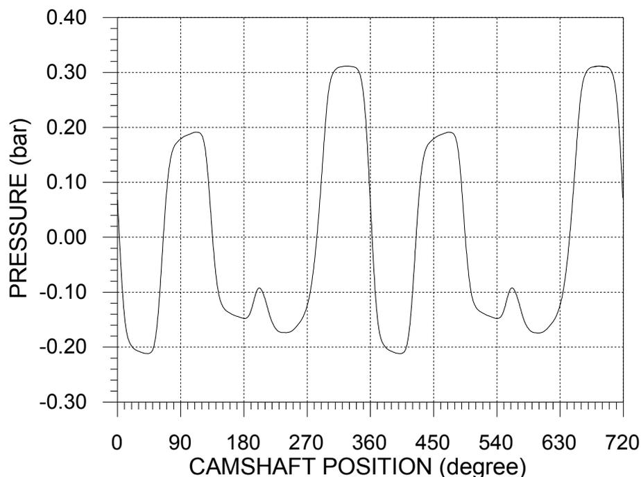
Figure 3 – Pressure fluctuation at 153 mm from the intake valve for 600 rev/min camshaft speed.
