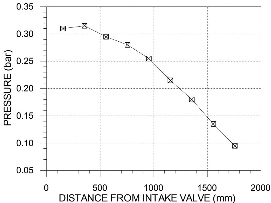
Figure 5 – Pressure fluctuation amplitude along the pipe for 2400 rev/min camshaft speed.
