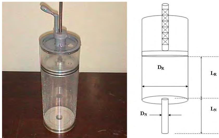
Figure 2 – Helmholtz resonator details.
