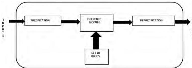
Figure 2. Schematic diagram of a Fuzzy Controller.
