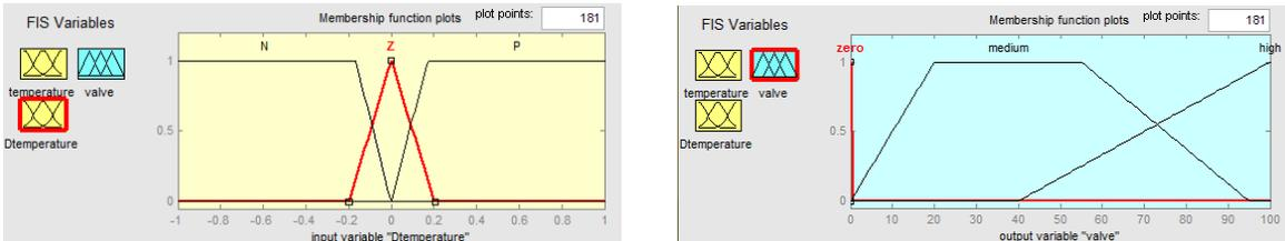
Figures 9 and 10. Membership functions to temperature derivative and percentage of valve opening.
