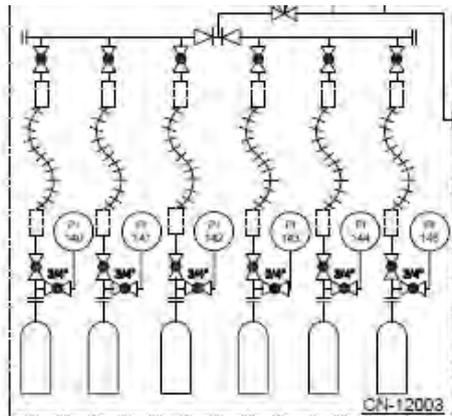
Figure 7. P&ID of carbon dioxide cylinders of the gas compression station.
