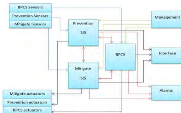
Figure 3. Control Architecture proposed for SIS Mitigation layer.
