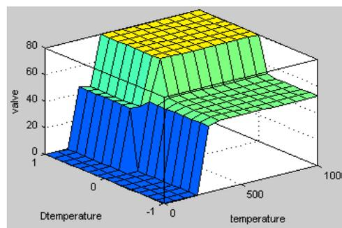
Figure 11. Surface generated by the fuzzy algorithm according to the fuzzy rules defined for the mitigation model.
