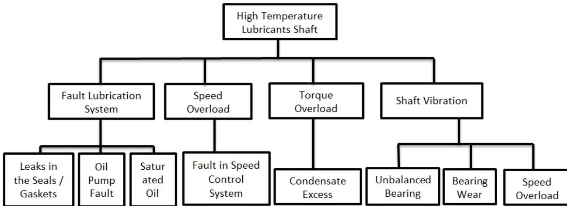
Figure 6. Suggested FTA for the top event “High Temperature Lubricants Shaft”
