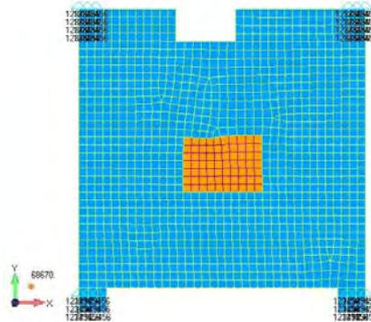
Figure 5. PCB board mesh, showing the supporting configuration and non-structural mass (orange).
