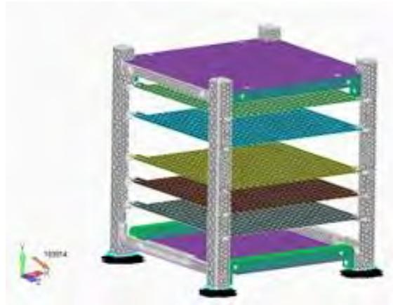
Figure 8. Mesh used in the analysis via FEMAP with NX NASTRAN.
