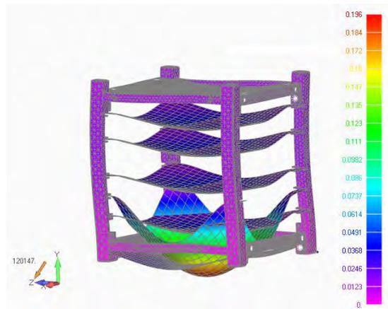
Figure 10. Displacement analysis, values in [mm].
