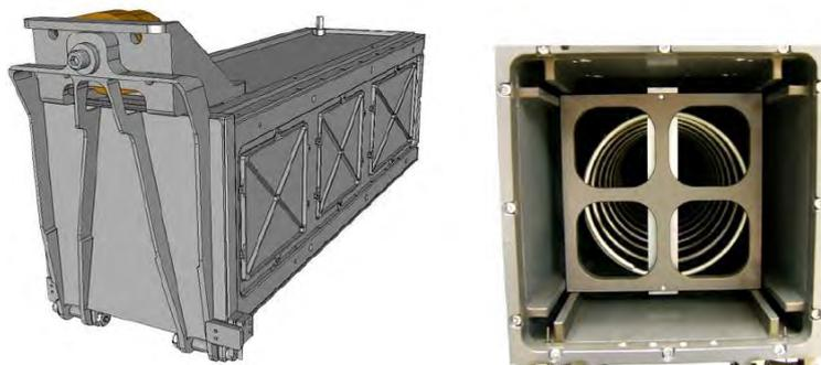
Figure 2. P-POD CAD model (left) and inside of a P-POD (right). From: CubeSat Design Specification, Rev. 12.
