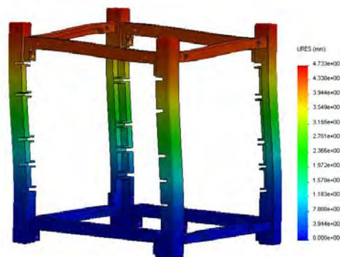
Figure 11. First mode of AESP-14 structure.
