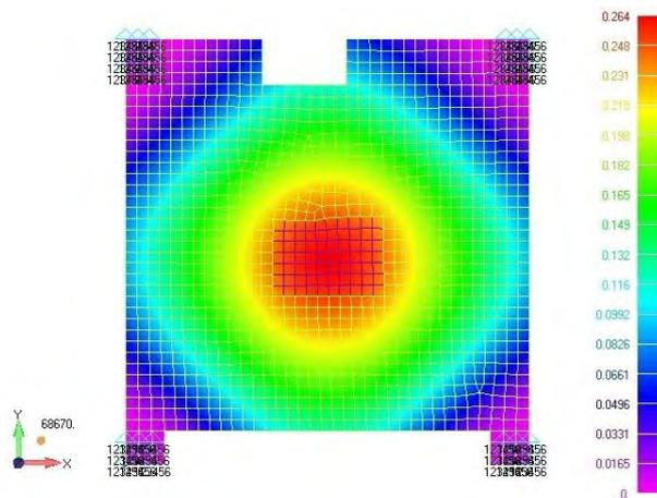
Figure 7. Analysis resultant displacement, values in [mm].
