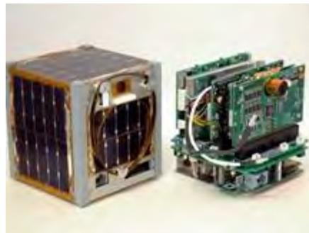
Figure 1. University of Tokyo Cubesat. From: <http://www.space.t.u-tokyo.ac.jp/cubesat/mission/V/index-e.html>
