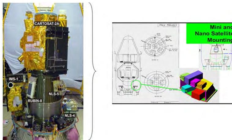
Figure 3. PODs attached to the Indian PSLV launcher mounting base. From: Raghava Murthy, D. V. A (2009).
