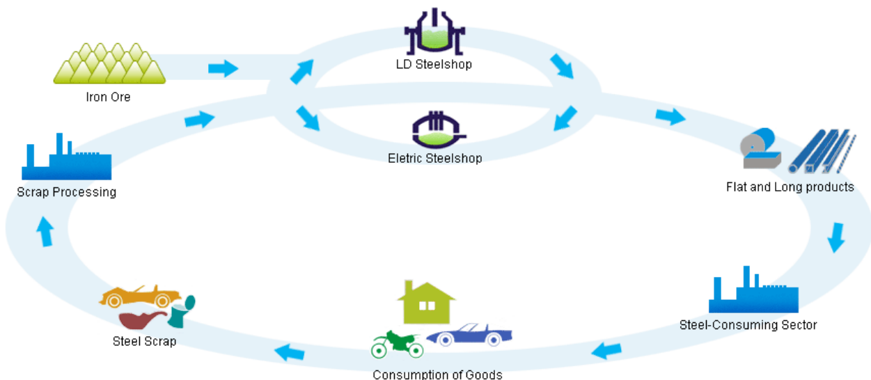
Figure 3. Steel recycling cycle (Institute of Steel, 2013)
