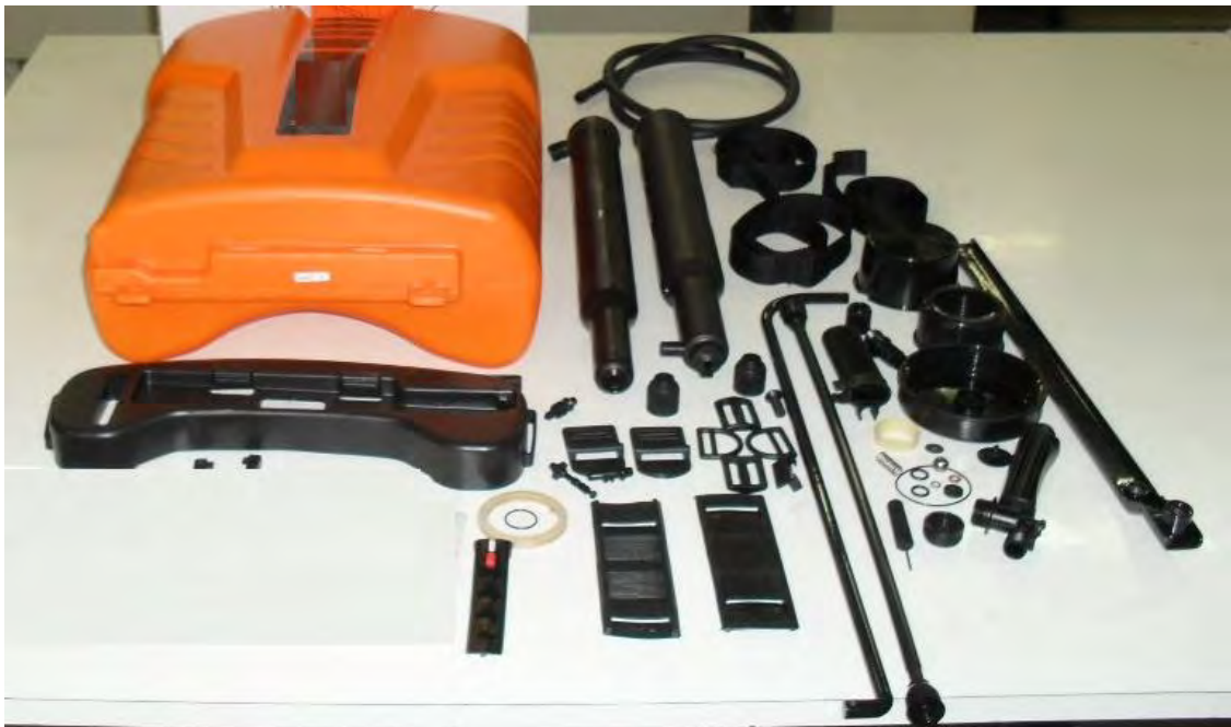
Figure 6. Knapsack Sprayer Components
