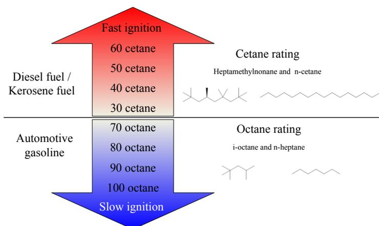
**Figure 1. Comparison between cetane and octane rating**
