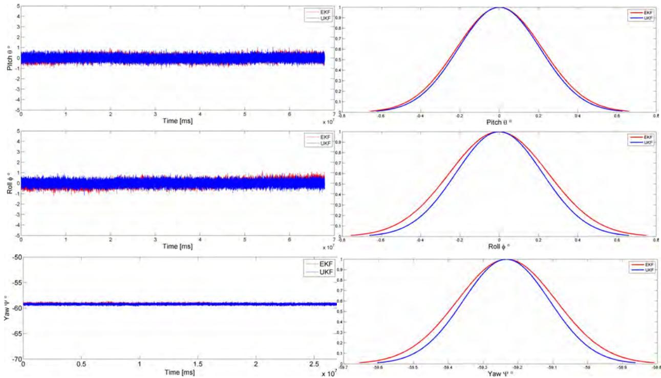
Figure 4. Estimated attitude of filters EKF and UKF in NED Frame
