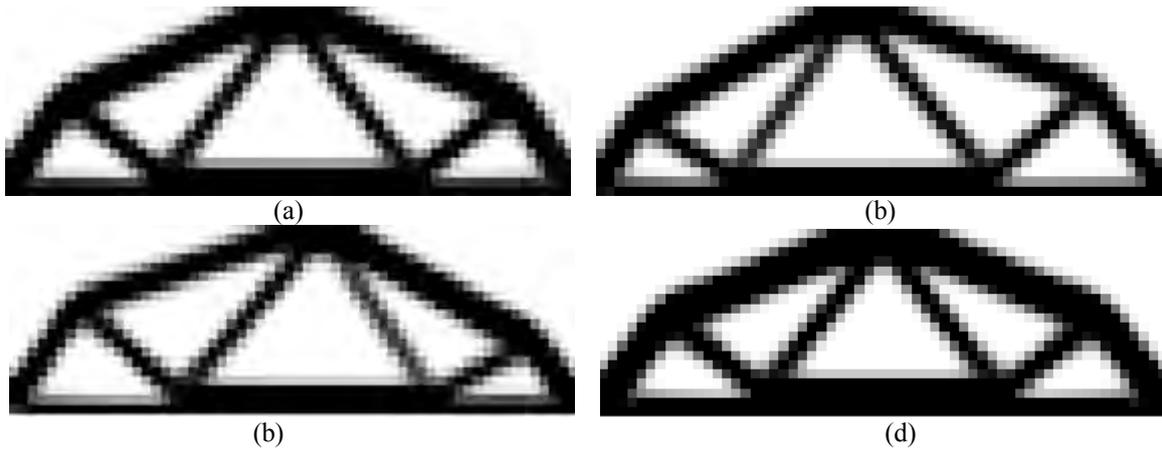
Figure 2 – (a) Model optimal topology, (b) Topology for the 4th Tree branch, (c) Topology for the 6th Tree branch and (d) Topology for the 26th Tree branch
