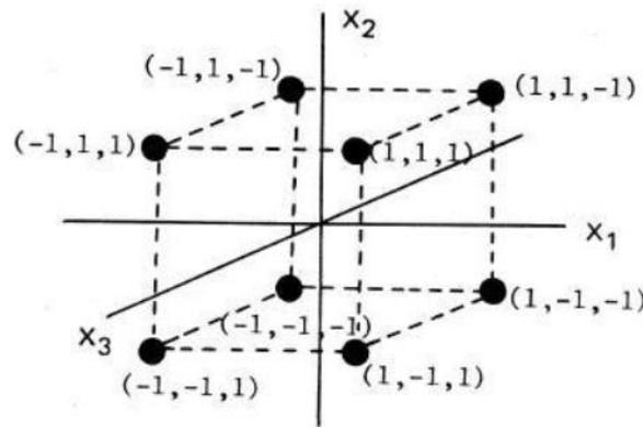
Figure 1 – Schematic drawing – interactions two level full factorial DOE with 3 parameters. Font: Noesis Solutions (2011)
