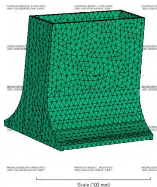
Figure 2. Creating the mesh in piece
