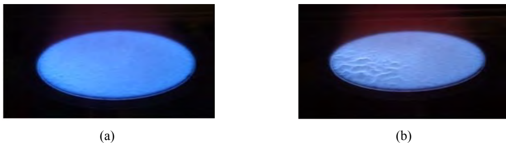
Figure 3. Pictures of the flame front obtained for premixed methane and air, with heat loss. (a) The flat flame and (b) the wrinkled flame.
