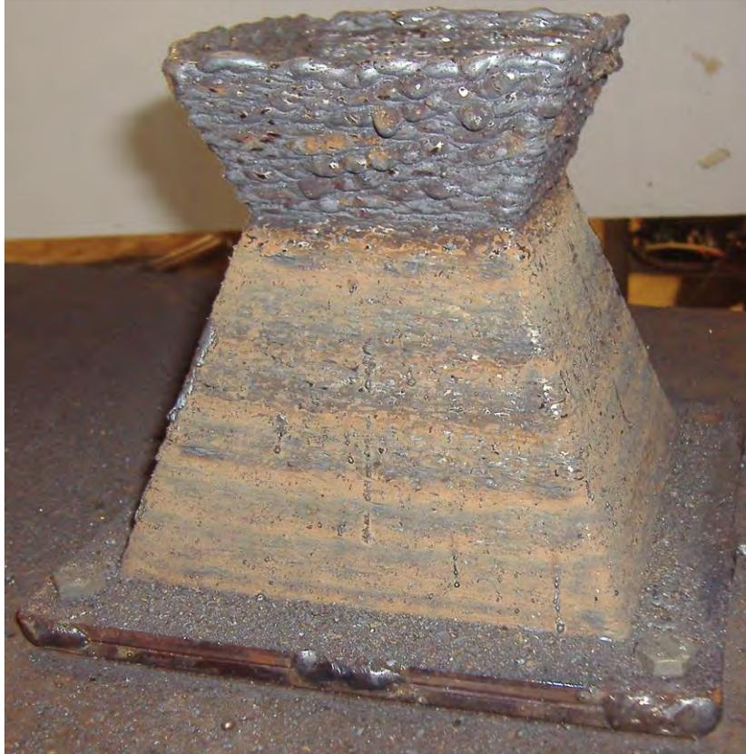
Figure 15. Deposited solid resulting of the primary deposition trial, before cleaning
