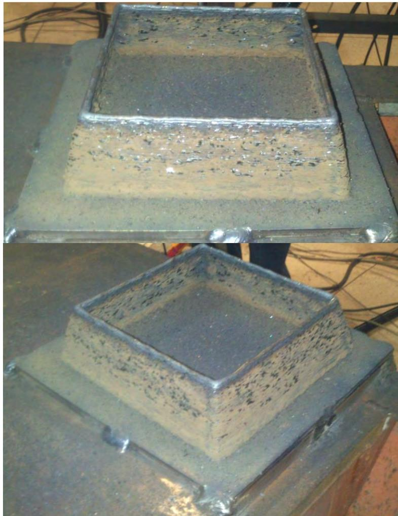
Figure 14. Views of the resulting deposited solid of auxiliary deposition trial 2, shortly after deposition
