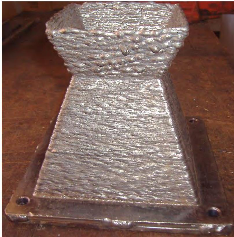
Figure 16. Deposited solid resulting of the primary deposition trial, after cleaning
