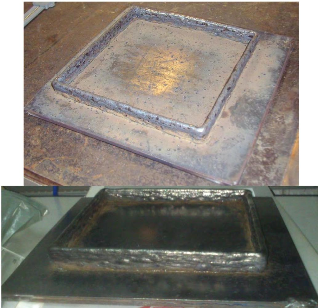
Figure 13. Views of the resulting deposited solid of auxiliary deposition trial 1, shortly after deposition (top) and after cleaning (bottom)
