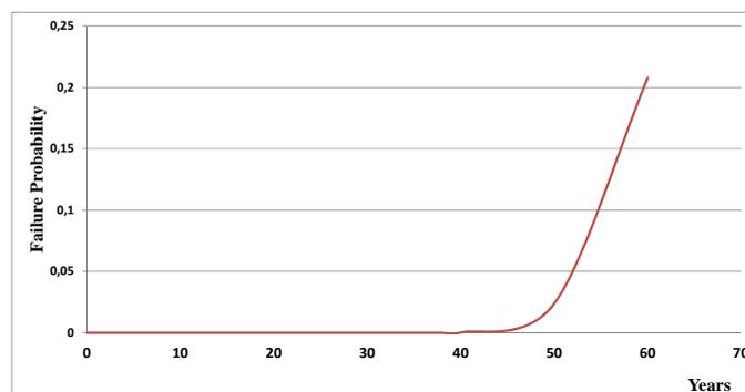
Figure 7. Probability of failure ( $P_F$ ) versus Exposure periods ( $T$ ) for 9.53mm pipe thickness
