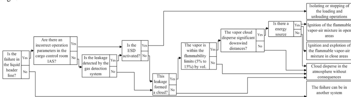
Figure 9. Cause-Consequence Diagram for the LNG leakage during loading and unloading operations
