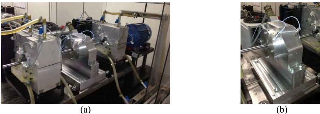
Figure 7. Configuration in the dynamic test: (a) general view of the test rig; (b) view of the active magnetic bearing (AMB).
