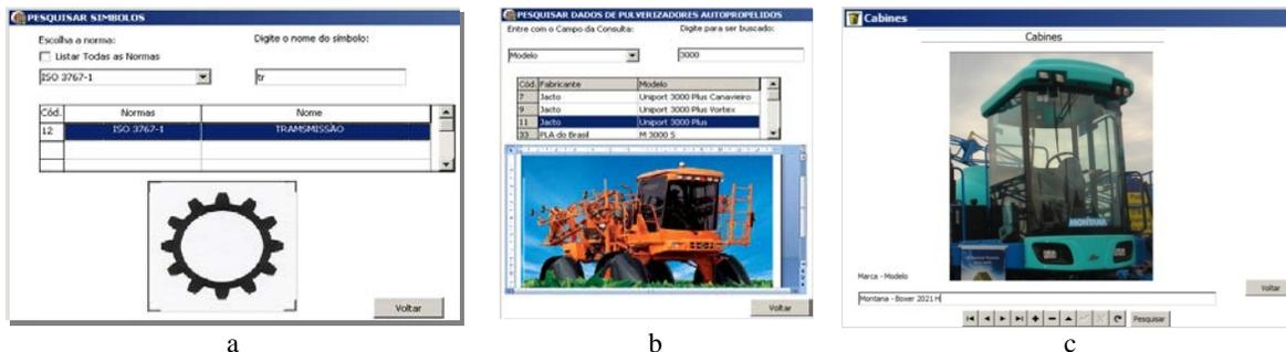
Figure 3. Interface SAPROC for searching graphic symbols (a), technical data of self-propelled sprayers (b) and cabins of agricultural machines (c)
