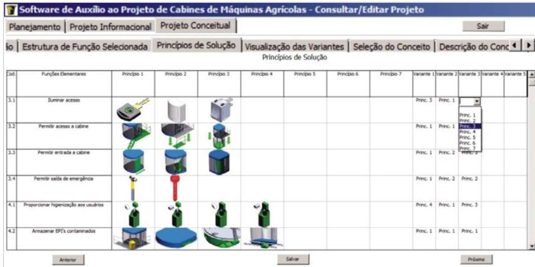
Figure 5. Interface SAPROC for tabs "Principles of Solution"
