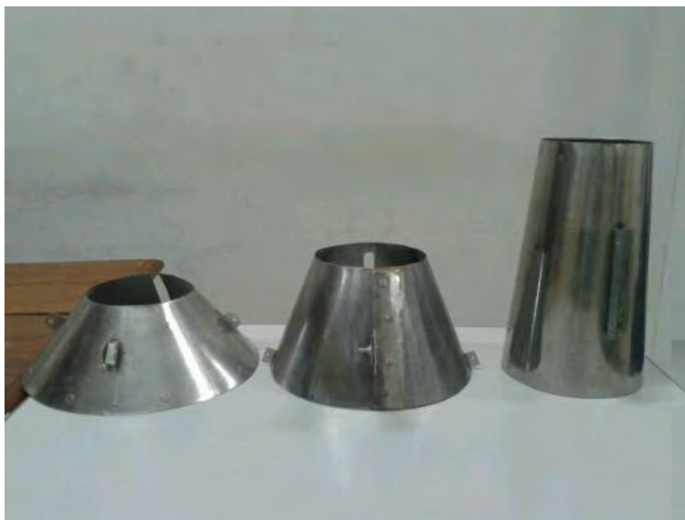
Figure 3. Diffusers used on the experimental study.
