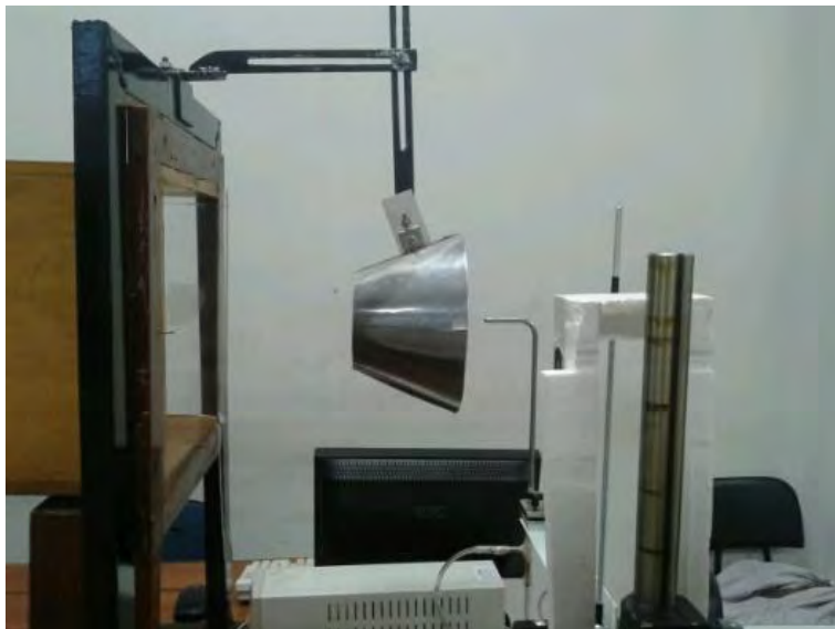
Figure 8. Diffuser positioned in front of the wind tunnel.
