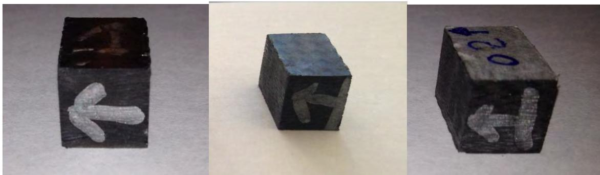
Figure 12. SHPB specimens  $(45^\circ,-45^\circ)_{21s}$  after test.
