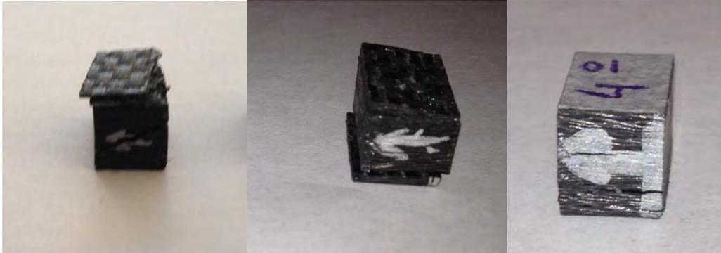
Figure 11. SHPB specimens  $(0^\circ,90^\circ)_{21s}$  after test.
