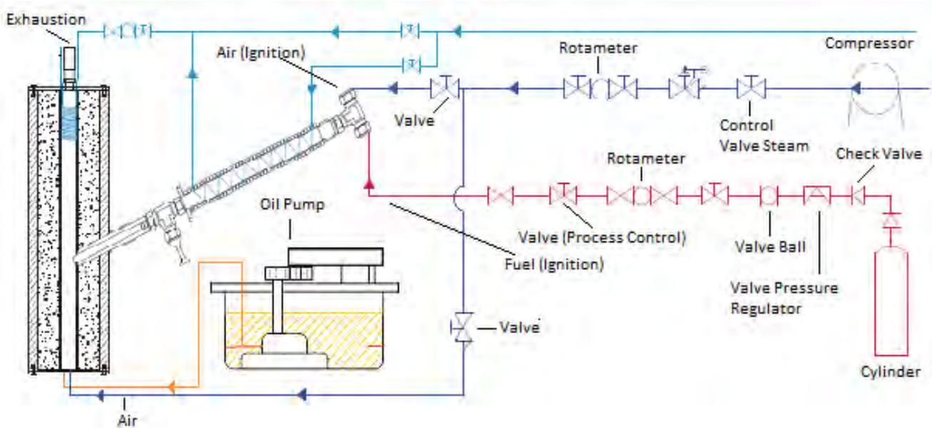
Figura 2 – Schematic diagram of operation supply system of GGPR
