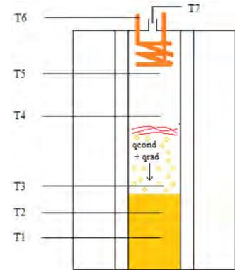
Figure 3: Schematic drawing of working principle of GGPR
