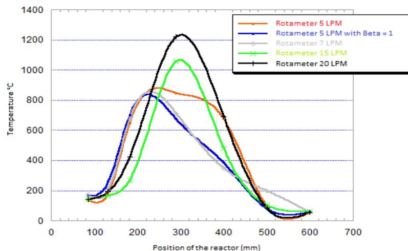
Figure 6: Temperature distribution profile along the GGPR's chamber for different air flow rate.
