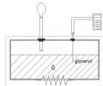
Figure 4: Auxiliary device for identifying gaseous compounds on the glycerol evaporation
