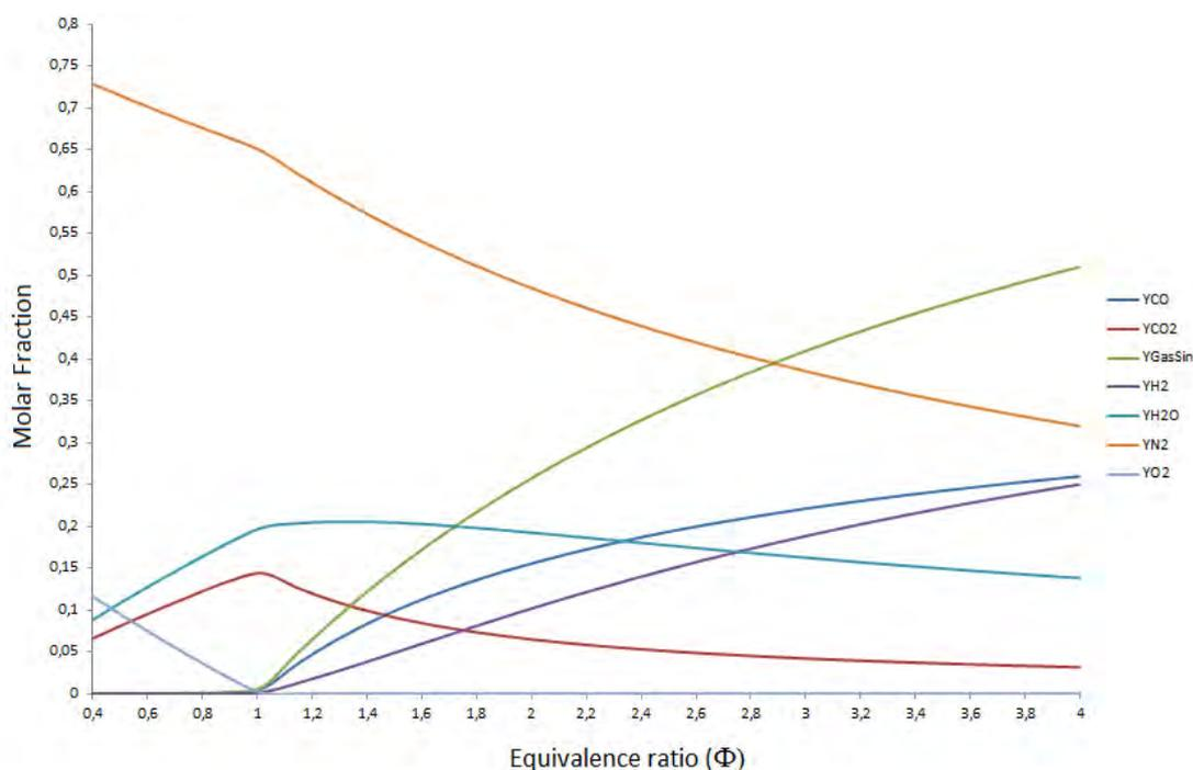
Figure 5 - Composition of the product stream as a function of equivalence ratio ( $\Phi$ ) in the state of chemical equilibrium.
