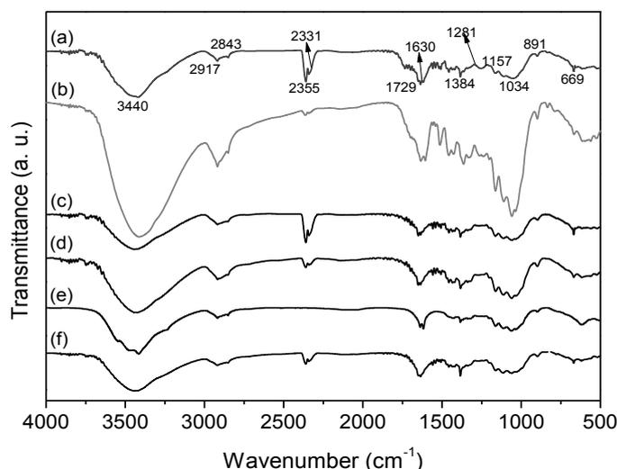
Figure 5. FTIR spectra of the sugarcane bagasse samples: (a) *in natura* and chemically pretreated: (b) 1% H<sub>2</sub>SO<sub>4</sub>; (c) 1% NaOH; (d) 2% NaOH; (e) 3% NaOH, and (f) 4% NaOH.
