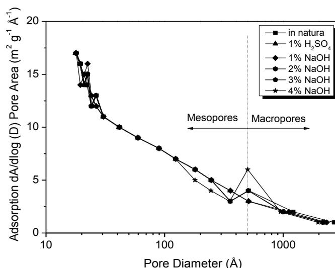
Figure 2. Distribution of pore diameter for *in natura* and chemically pretreated sugarcane bagasse samples.
