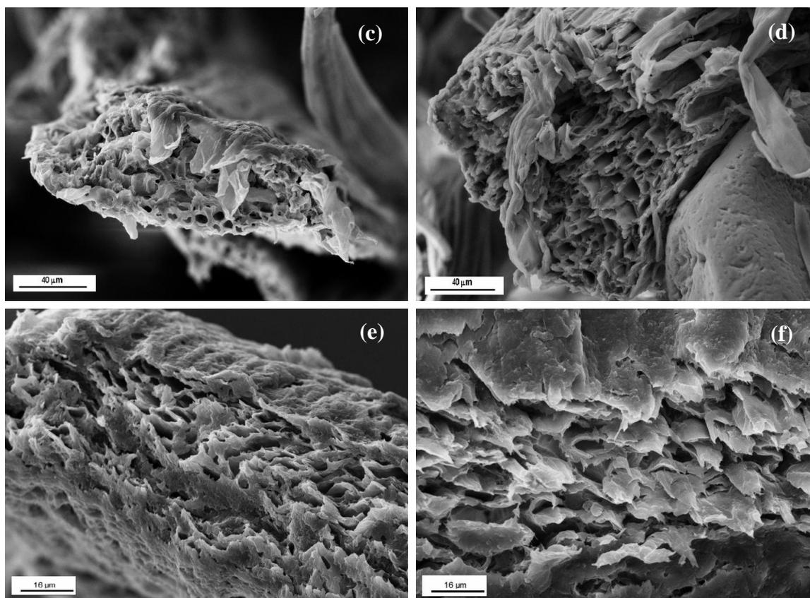
Figure 4. SEM micrographics of the cross-section of sugarcane bagasse fibers: (a) *in natura* (750 x) and chemically pretreated: (b) 1% H<sub>2</sub>SO<sub>4</sub> (1,500 x); (c) 1% NaOH (1,000 x); (d) 2% NaOH (1,000 x); (e) 3% NaOH (2,000 x), and (f) 4% NaOH (2,000 x).
