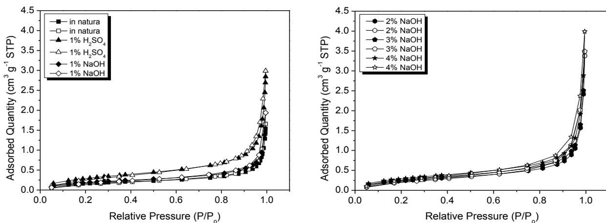
Figure 1. Adsorption and desorption isotherms in nitrogen gas for the sugarcane bagasse samples *in natura* and chemically pretreated. Full symbols indicate adsorbed and empty symbols desorbed quantity.
