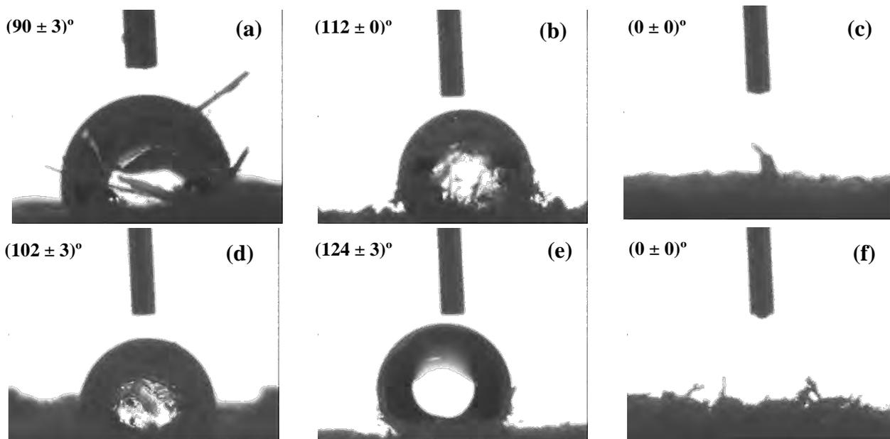
Figure 6. Contact angles of the sugarcane bagasse samples (a) *in natura* and chemically pretreated: (b) 1% H<sub>2</sub>SO<sub>4</sub>; (c) 1% NaOH; (d) 2% NaOH; (e) 3% NaOH, and (f) 4% NaOH.
