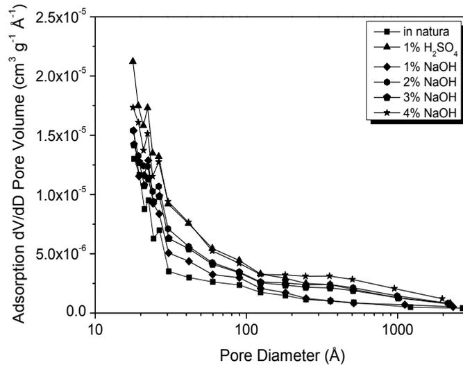
Figure 3. Distribution of pore volume for *in natura* and chemically pretreated sugarcane bagasse samples.
