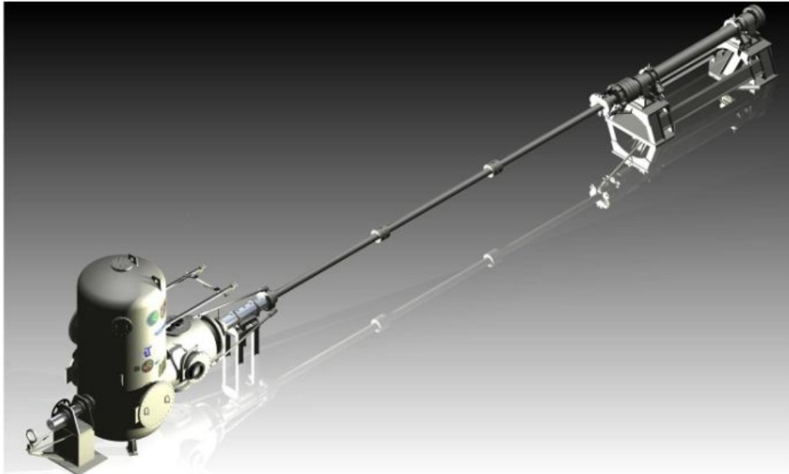
Figure 17: T3 0.60-m. nozzle exit diameter Hypersonic Shock Tunnel.
