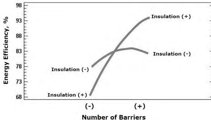
Figure 5. Effects of the interaction between insulation II and the number of radiant barriers.
