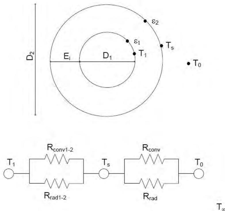
Figure 1. Design of the physical system and the thermal circuit describing the simple reflective insulation configuration.
