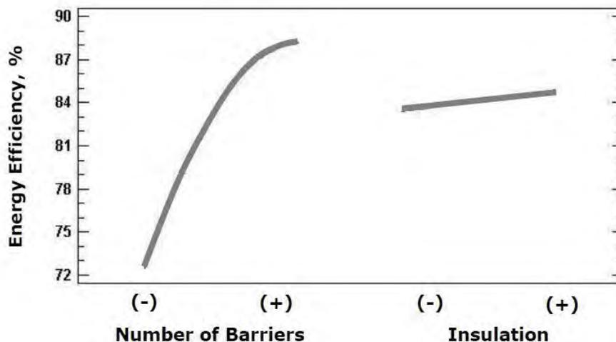
Figure 4. Inherent effects of insulation II and the number of radiant barriers.
