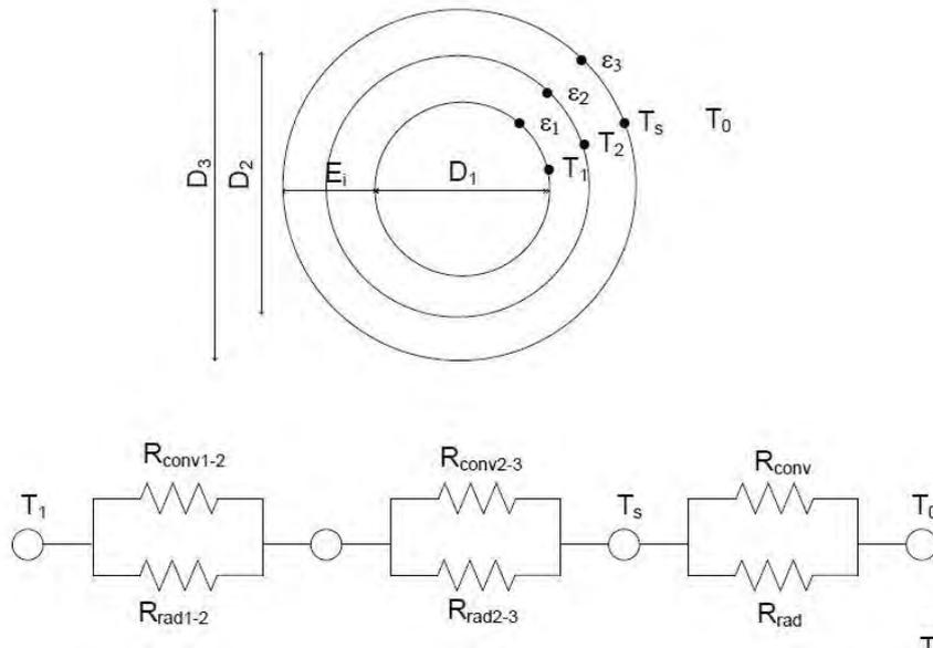
Figure 2. Design of the physical system and the thermal circuit describing the double reflective insulation configuration.
