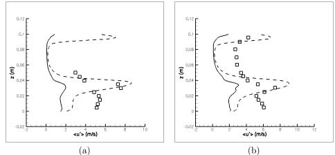
Figure 2. Mean velocity fluctuations, obtained from the application of the turbulence models proposed by Smagorinsky (1963) and Germano *et al.* (1991): (a)  $x_m = 0.08 m$  and (b)  $x_m = 0.10 m$ .  $\Box$  Moreau *et al.* (1996), — Classical Smagorinsky's model and - - Dynamic Smagorinsky's model.
