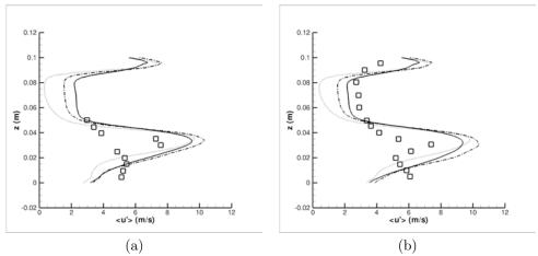
Figure 10. Mean velocity fluctuations obtained from the application of the turbulence model proposed by Germano *et al.* (1991) and the use of SEM and RFG methods for the inlet turbulent conditions: (a)  $x_m = 0.08$  m and (b)  $x_m = 0.10 \text{ m}$ .  $\Box$  Moreau *et al.* (1996), — RFG, … SEM - case B, - - - SEM - case D.
