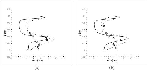
Figure 4. Mean velocity fluctuations obtained from the application of the turbulence model proposed by Germano *et al.* (1991) and the RFG method for the inlet turbulent conditions: (a)  $x_m = 0.08 \ m$  and (b)  $x_m = 0.10 \ m$ .  $\Box$  Moreau *et al.* (1996), — Dynamic Smagorinsky's model and - - Dynamic Smagorinsky's model with RFG.
