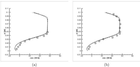
Figure 9. Mean velocity profiles obtained from the application of the turbulence model proposed by Germano et al. (1991) and the use of SEM and RFG methods for the turbulent inlet conditions: (a)  $x_m = 0.08 \ m$  and (b)  $x_m = 0.10 \ m$ .  $\Box$  Moreau et al. (1996), — RFG, … SEM - case B, - · - SEM - case D.
