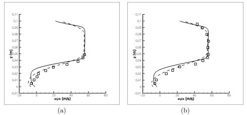
Figure 3. Mean velocity profiles obtained from the application of the turbulence model proposed by Germano *et al.* (1991) and the RFG method for the inlet turbulent conditions: (a)  $x_m = 0.08 \ m$  and (b)  $x_m = 0.10 \ m$ .  $\Box$  Moreau *et al.* (1996), — Dynamic Smagorinsky's model and - - Dynamic Smagorinsky's model with RFG.
