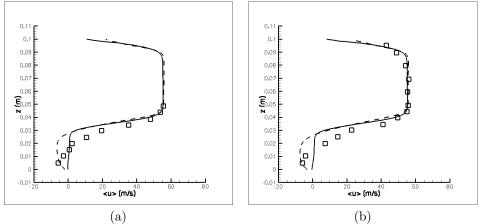
Figure 1. Mean velocity profiles obtained from the application of the turbulence models proposed by Smagorinsky (1963) and Germano *et al.* (1991): (a)  $x_m = 0.08 \ m$  and (b)  $x_m = 0.10 \ m$ .  $\Box$  Moreau *et al.* (1996), — Classical Smagorinsky's model and - - - Dynamic Smagorinsky's model.
