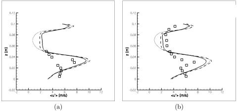
Figure 8. Mean velocity fluctuations obtained from the application of the turbulence model proposed by Germano *et al.* (1991) and the use of SEM and RFG methods for the inlet turbulent conditions: (a)  $x_m = 0.08 m$  and (b)  $x_m = 0.10 m$ .  $\Box$  Moreau *et al.* (1996), — RFG, - - SEM - 10000 eddies, - - SEM - 100000 eddies.
