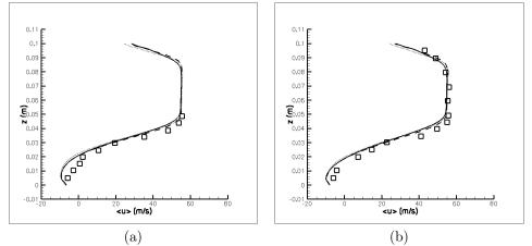
Figure 7. Mean velocity profiles obtained from the application of the turbulence model proposed by Germano et al. (1991) and the use of SEM and RFG methods for the turbulent inlet conditions: (a)  $x_m = 0.08 \ m$  and (b)  $x_m = 0.10 \ m$ .  $\Box$  Moreau et al. (1996), — RFG, - - SEM - 10000 eddies, - - SEM - 10000 eddies.
