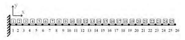
Figure 4. Beam modeled with 25 finite elements
