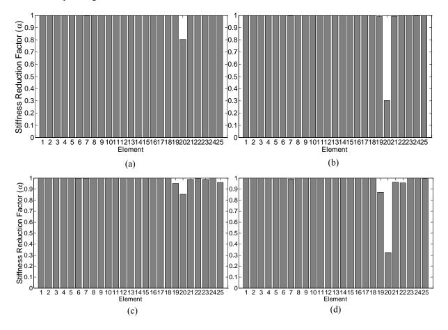
Figure 5. Free vibration and 3% noise: (a) Damage Scenario 1 through the P-NMA, (b) Damage Scenario 2 through the P-NMA, (c) Damage Scenario 1 with HS (Fadel Miguel *et al.*, 2012), (d) Damage Scenario 2 with HS (Fadel Miguel *et al.*, 2012).
