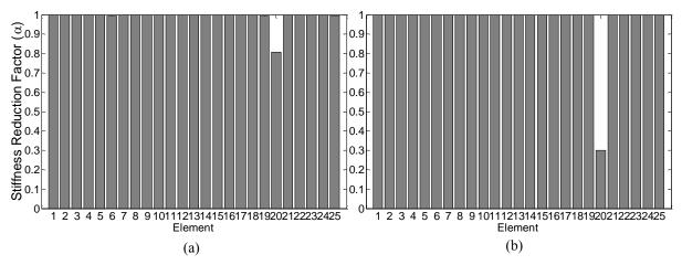
Figure 6: Free vibration and 5% noise through the P-NMA: (a) Damage Scenario 1, (b) Damage Scenario 2.
