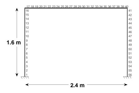
Figure 1. Portal plane frame modeled with 56 finite elements
