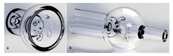
Figure 2. Enhanced geometry of the jet stirred reactor
