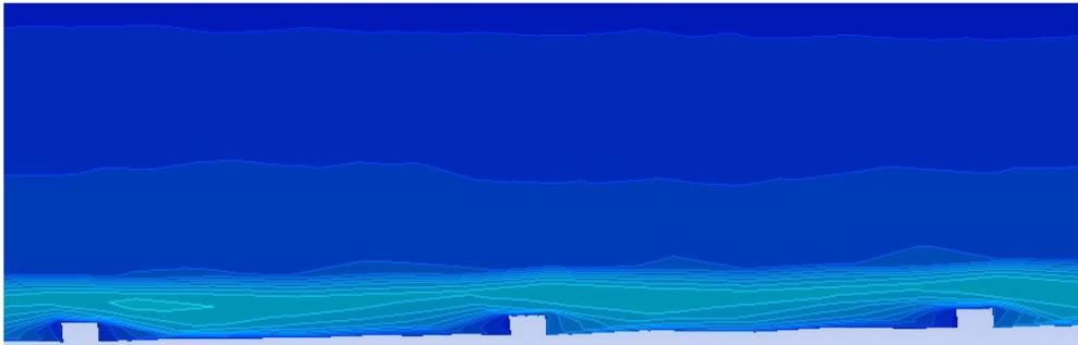
Figure 11: Turbulence kinetic energy on near wall region.
