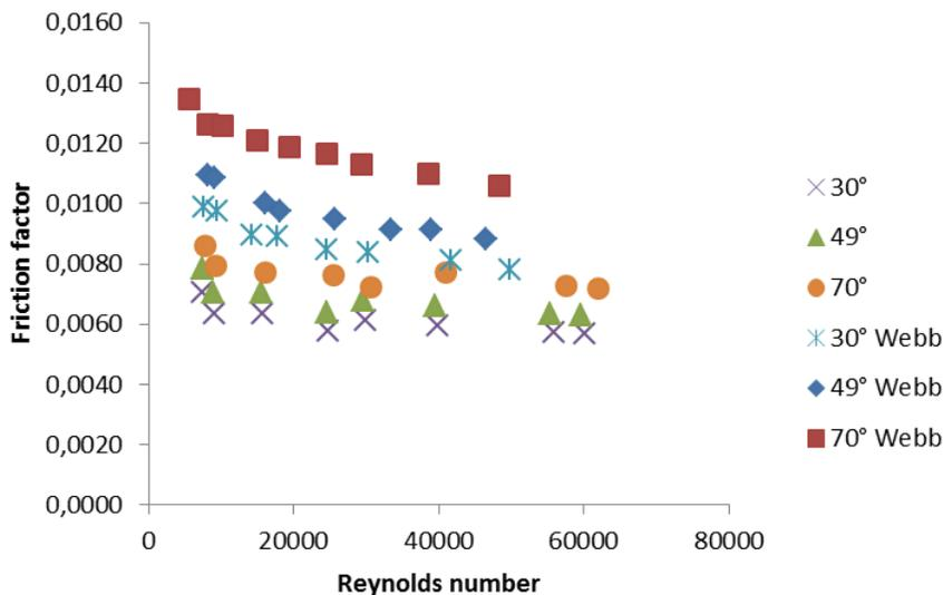
Figure 10: Friction factor vs. Reynolds number numerical results.
