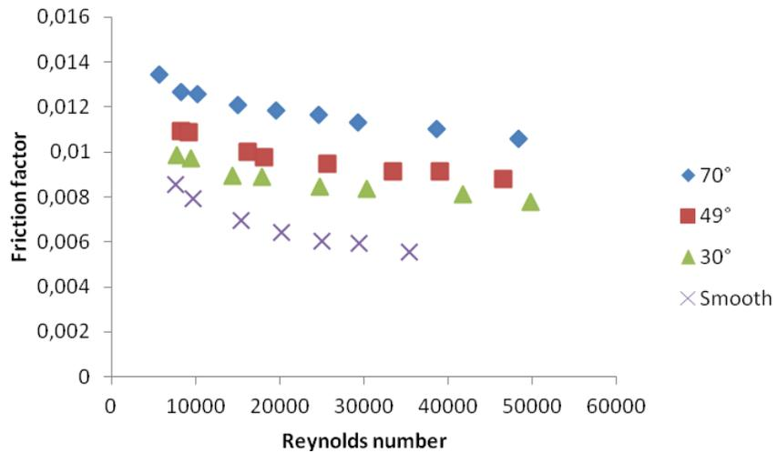
Figure 4: Friction factor vs. Reynolds number for tested ribs helix angles studied by Webb et al. (1980)
