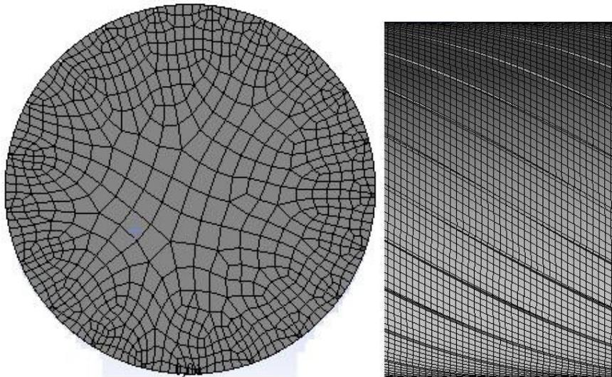
Figure 8: Mesh adopted on numerical simulations.
