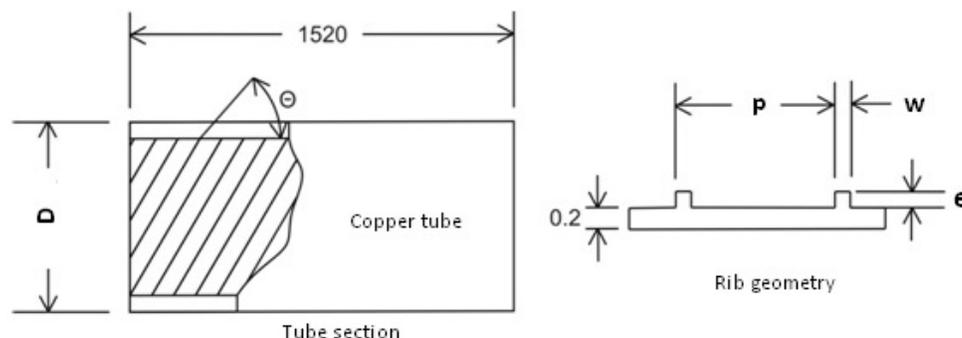
Figure 2: Helically rib-roughened tube used by Webb et al. (1980).
