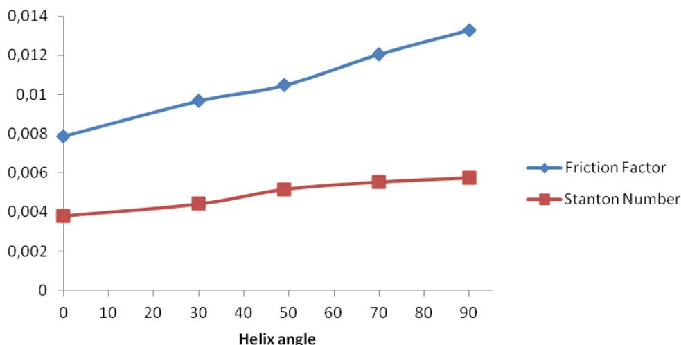
Figure 5: Friction factor and Stanton number vs. helix angle for  $Re=10000$ .
