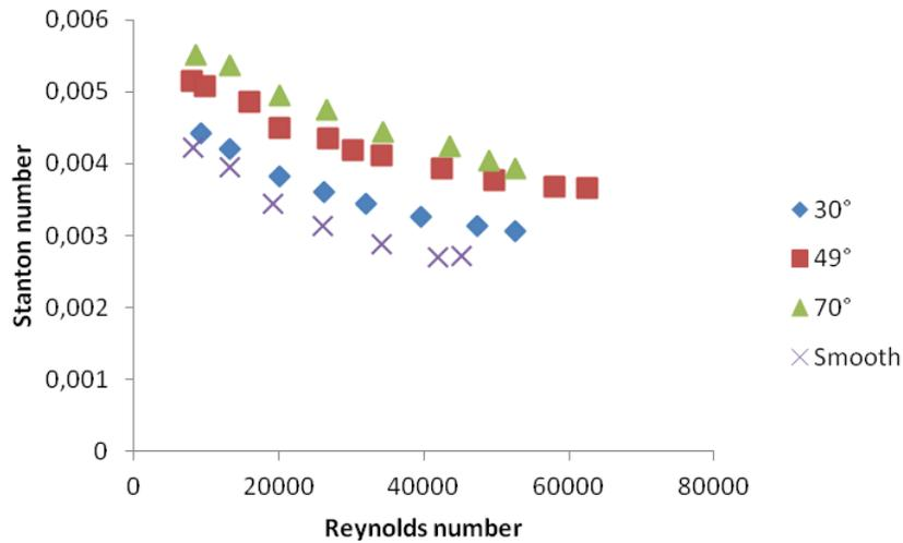
Figure 3: Stanton number vs. Reynolds number for tested ribs helix angles studied by Webb et al. (1980)
