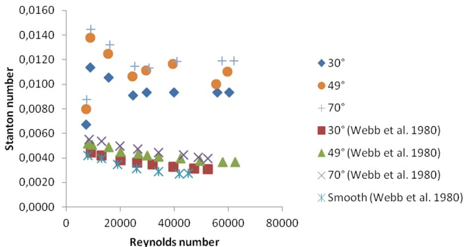
Figure 9: Stanton number vs. Reynolds number numerical results.
