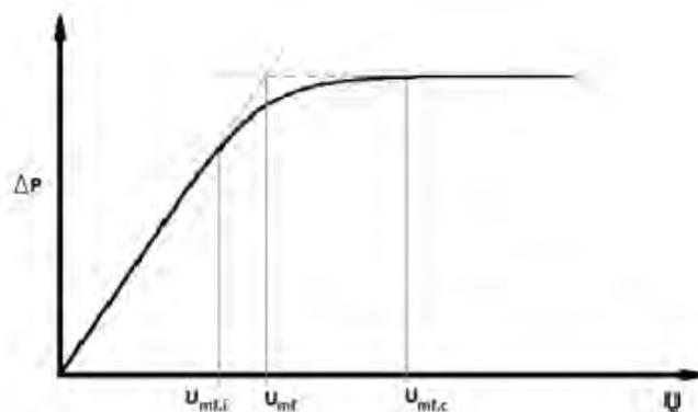
Figure 2. Typical curve of pressure drop versus superficial velocity for mixtures
