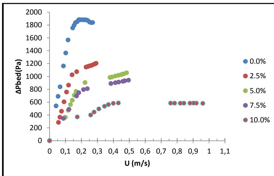
Figure 4. Pressure drop versus superficial velocity of bamboo-sand mixtures
