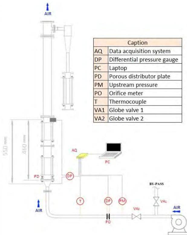
(b) Schematics of the experimental set up
