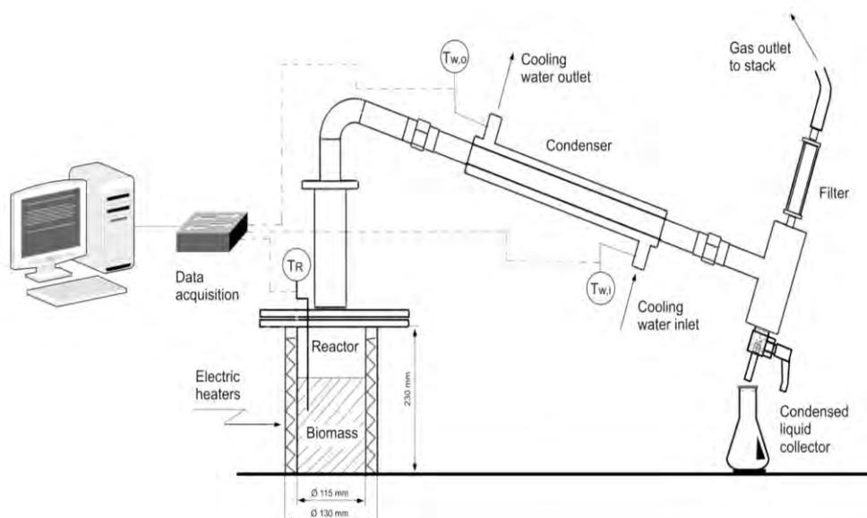
Figure 3. Fixed bed pyrolysis system.
