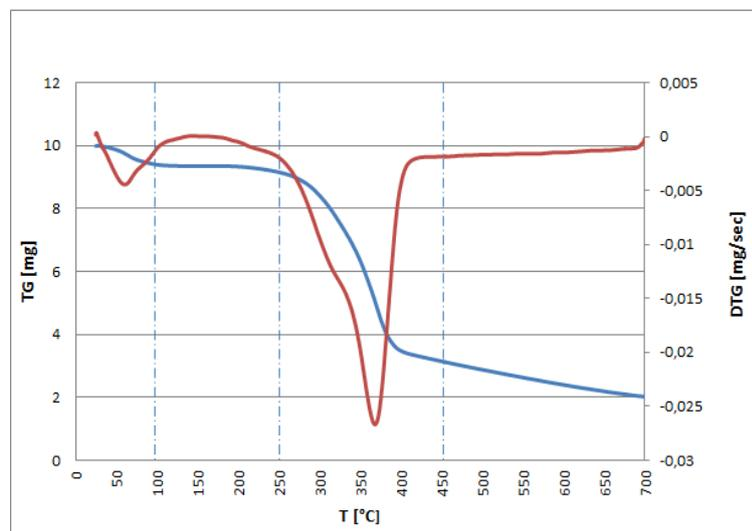
Figure 5. The TG curve of bamboo pyrolysis
