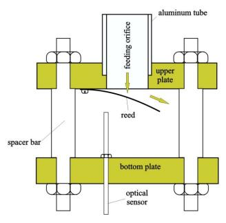
Figure 2 – Test section
