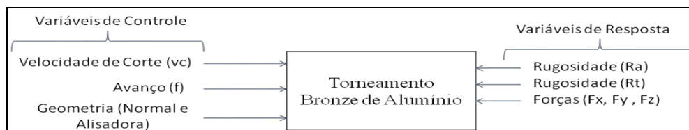
Figure 3 - Process Turning Bronze Aluminum Source: Paiva, 2010 (adapted by the author).
