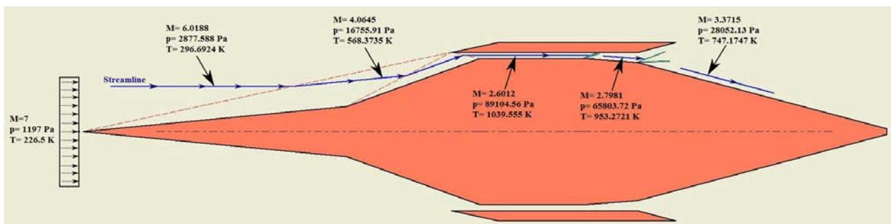
Figure 8: Analytical Theoretical Analysis applied to the VHA 14-X S at 30km altitude Mach number 7.
