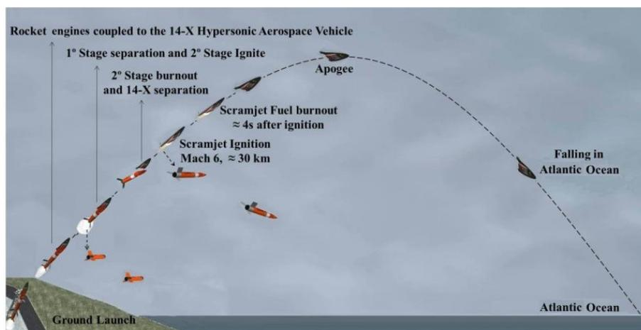
Figure 3: Hypersonic Accelerator Vehicle and 14-X Hypersonic Aerospace Vehicle in ballistic trajectory.
