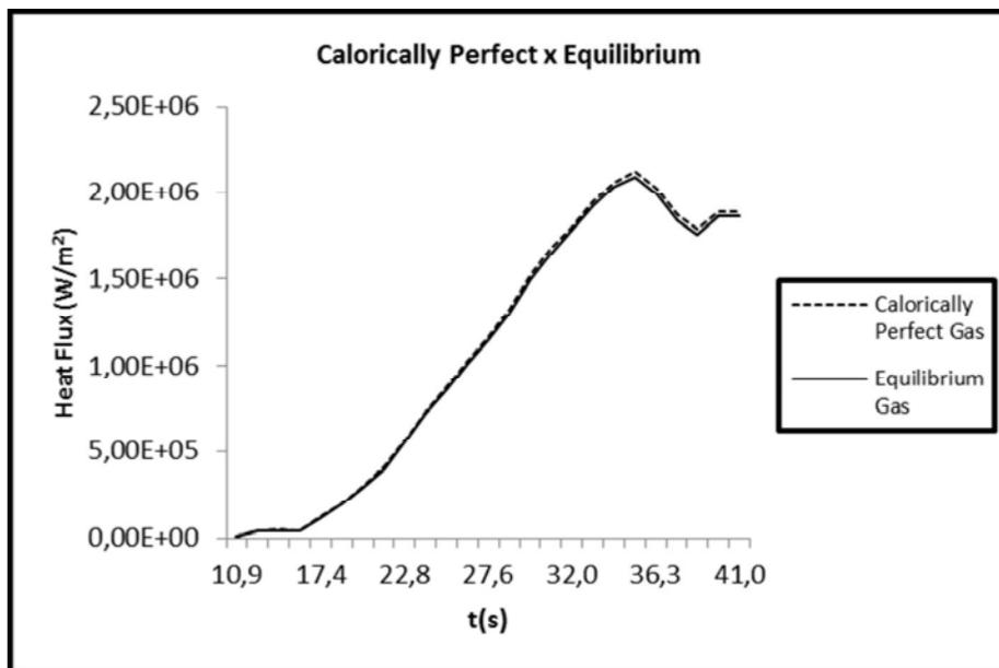
Figure 9: heat flux in the stagnation point of vehicle calorically perfect gas x equilibrium.
