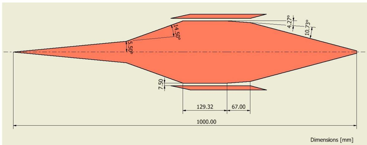
Figure 5: Dimensional for the VHA 14-X S.
