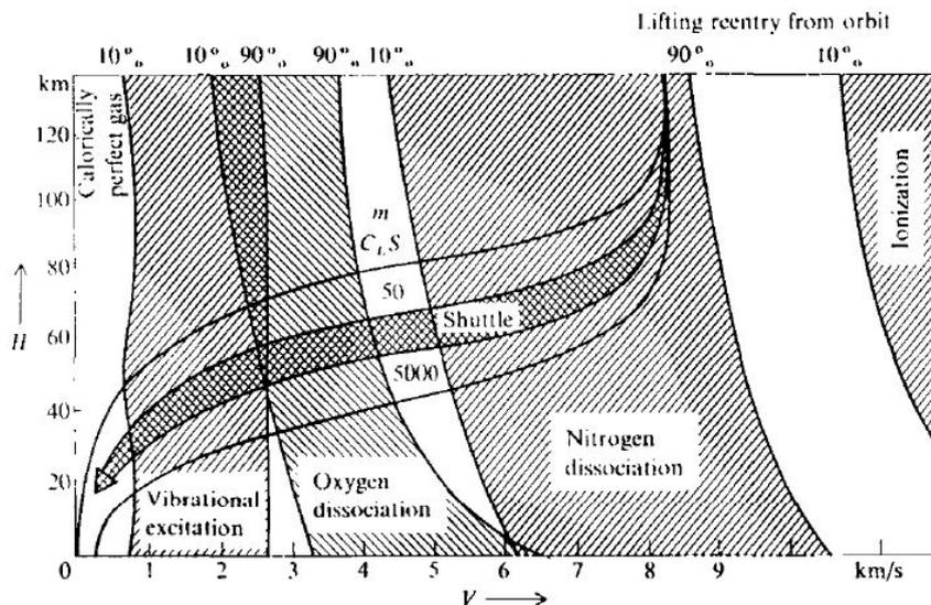
Figure 10: Velocity map with superimposed regions of vibration, excitation, dissociation and ionization.
