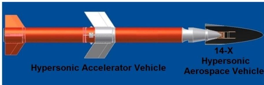
Figure 2: Hypersonic Accelerator Vehicle and 14-X Hypersonic Aerospace Vehicle coupled.
