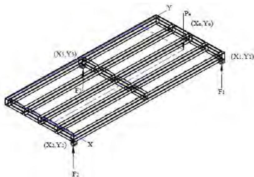
Figure 4. Positioning of the load cells in the left force platform.
