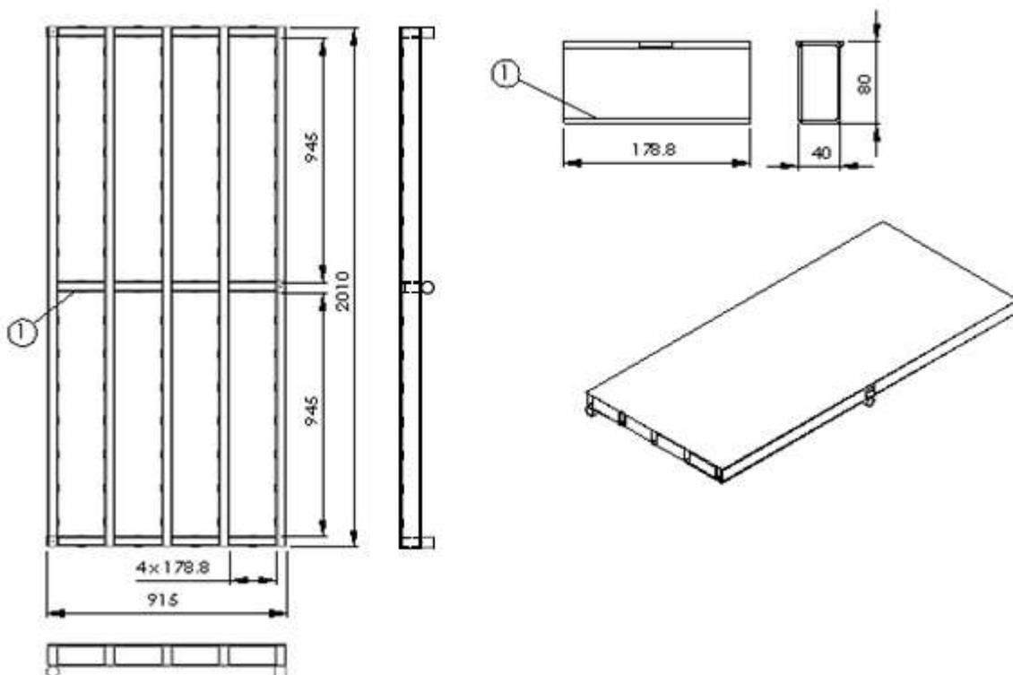
Figure 1. The main dimensions of the force platform.
