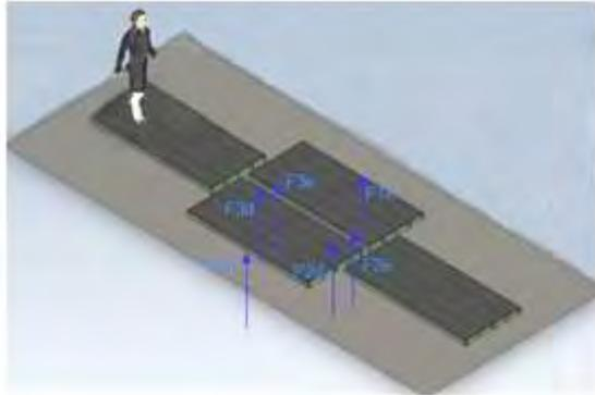
Figure 2. Model of force platform for gait analysis (blue arrows means force reaction from load cells).
