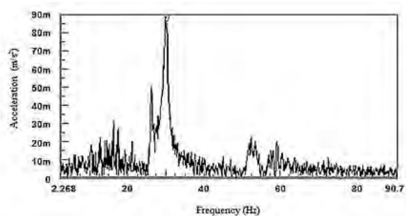
Figure 5. Acceleration frequency spectrum.
