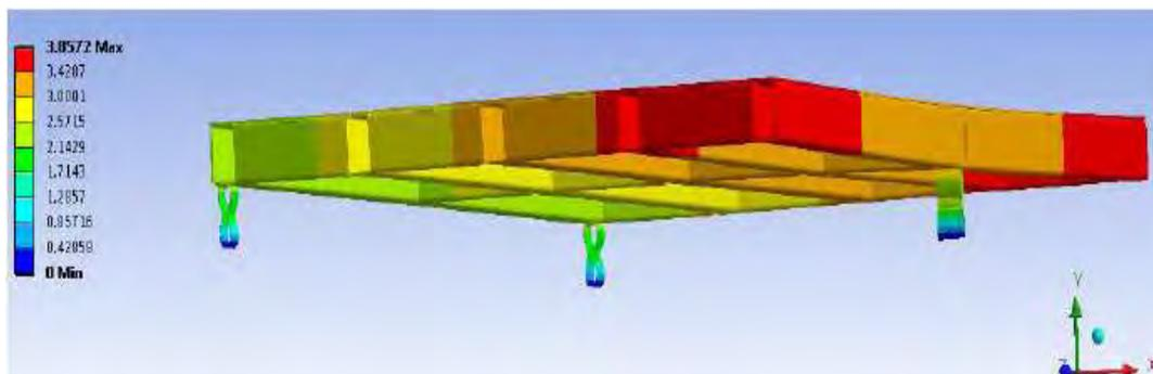
Figure 7. First vibration mode of the force platform.
