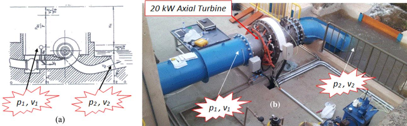
Figure 7. Turbine measuring points; (a): IEC 60091 turbine measuring points, (b): 20 kW Machine during the test (courtesy of Hydrel, May 8<sup>st</sup> 2013)
