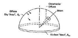
Figure 2. Components of diffuse radiation (Duffie and Beckman, 2006)
