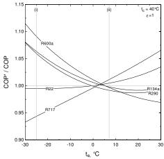
Figura 9. COP variation in case of constrained capacity for an IHX with  $\epsilon$ =1
