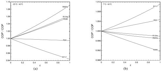
Figure 8. COP variation in case of constrained capacity: (a)  $t_e$ =-25°C and (b)  $t_e$ =7°C ( $t_c$ =40°C)
