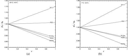
Figure 5. Evaporating pressure variation in case of constrained capacity: (a)  $t_e$ =-25°C and (b)  $t_e$ =7°C ( $t_c$ =40°C)
