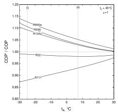
Figure 4. COP variation in case of constrained pressures for  $\varepsilon$ =1
