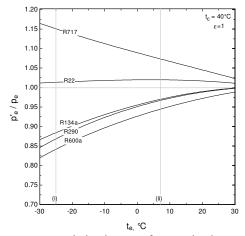
Figure 6. Evaporating pressure variation in case of constrained pressures for an IHX with  $\epsilon$ =1
