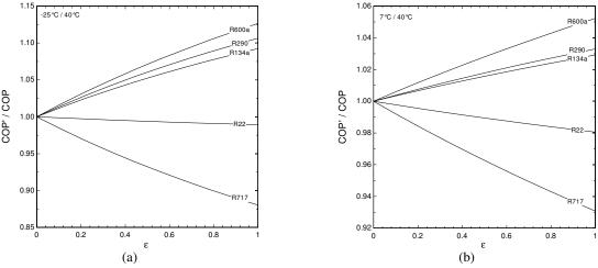
Figure 3. COP variation in case of constrained pressures: (a)  $t_e$ =-25°C and (b)  $t_e$ =7°C ( $t_c$ =40°C)
