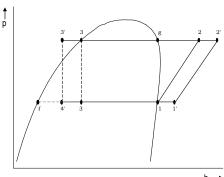
Figura 2. Thermodynamic representation of the refrigeration cycles under analysis in a p-h diagram
