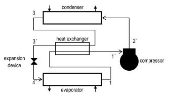
Figure 1. Schematic of the refrigeration cycle employing an internal heat exchanger
