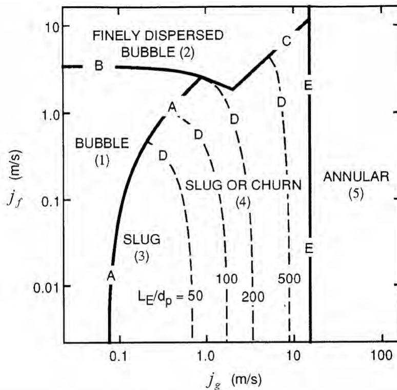
Figure 3. Taitel & Dukler regime map for upward gas-liquid flows -  $D = 50 \text{ mm}$  (Taitel *et al.*, 1980).
