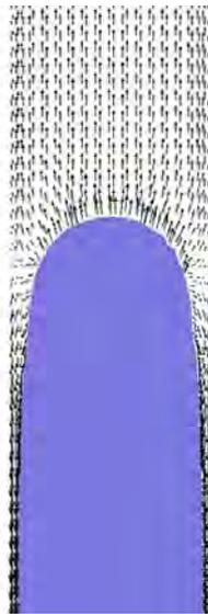
Figure 7. Velocity vectors of water flow around the nose of a Taylor bubble.
