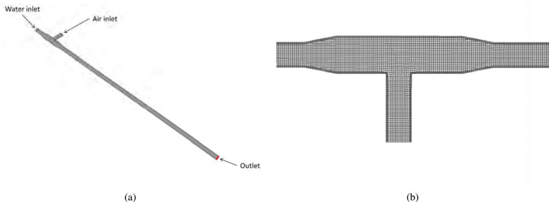
Figure 5. (a) Mixer with tube geometry; (b) hexahedral mesh of the mixer region.
