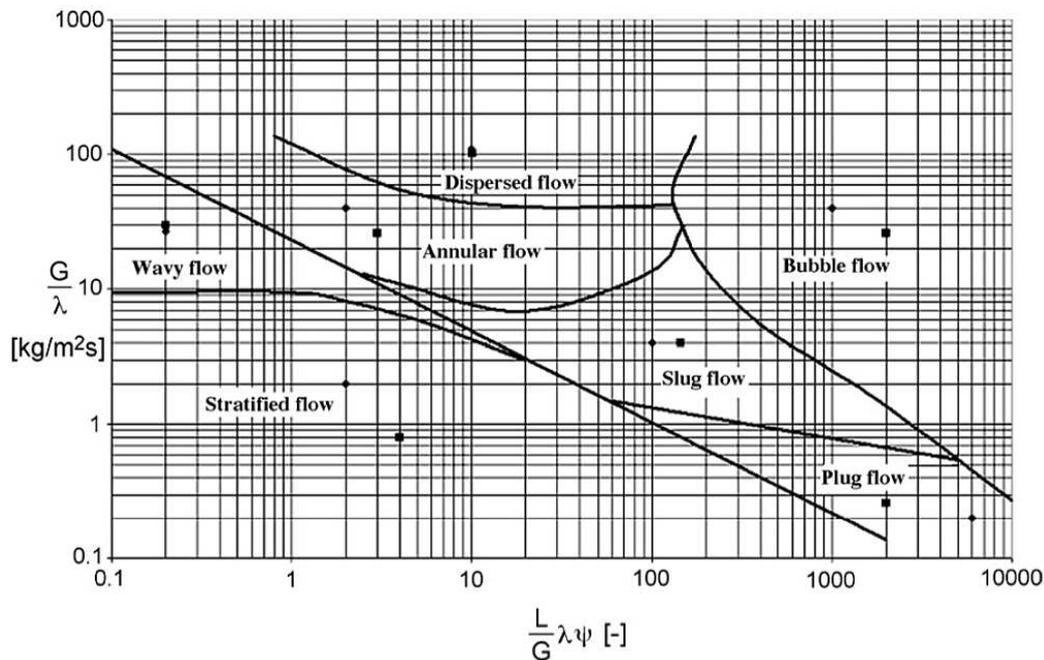
Figure 2. Baker chart (extracted from (De Schepper *et al.*, 2008)).
