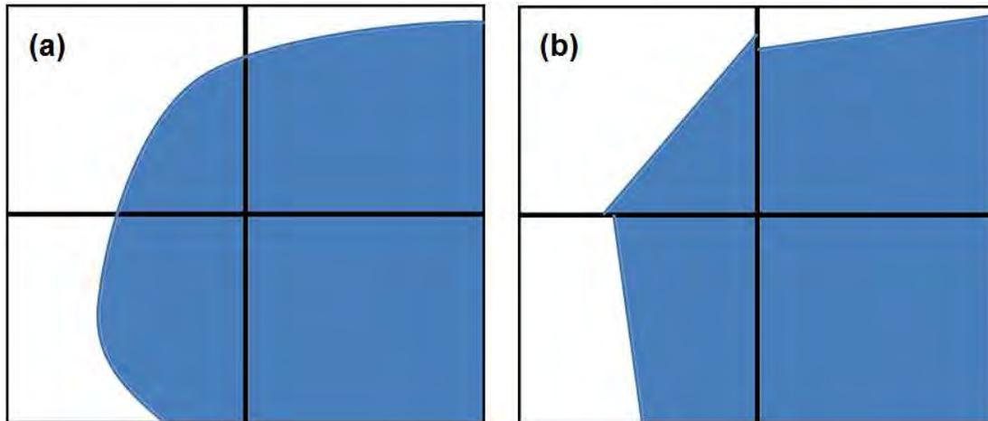
Figure 4. Interface reconstruction: (a) actual interface shape, (b) interface reconstructed through PLIC algorithm.
