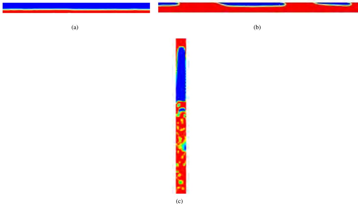
Figure 6. Water volume fractions of calculated air-water regimes: (a) stratified; (b) horizontal plug; (c) vertical slug (operational conditions in Tab. 2. Blue color means 100% air, red color represents 100% water.
