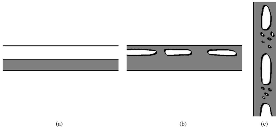
Figure 1. Representation of flow regimes: (a) stratified; (b) horizontal plug; (c) vertical slug - Grey color represents liquid phase and white color represents gas phase.
