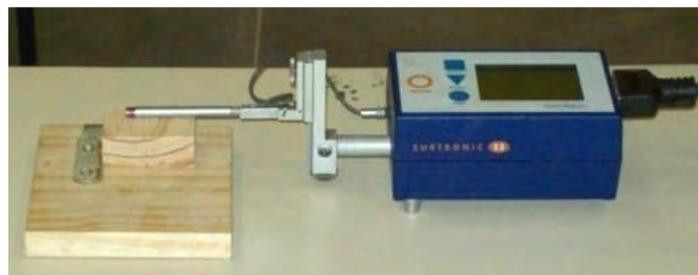
Figure 4 - TAYLOR HOBSON rugosimeter brand, model Surtronic 25 +.
