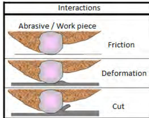
Figure 1 - Schematic representation of the interactions of the abrasive tool with the piece-work. (SUBRAMANIAN, K. apud GONÇALVES *et al.*)
