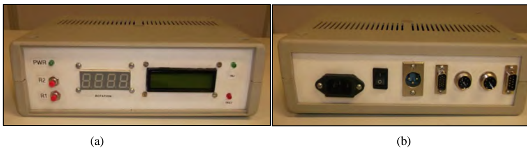
Figure 2. Front (a) and back (b) views of ECU case.
