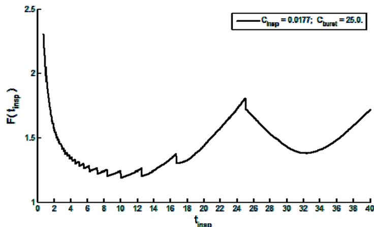
Figure 1 - Objective function values for different times between inspections, reference cost configuration.
