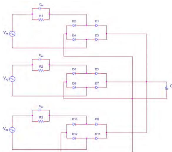
Figure 7. Schematic diagram simulating the full-bridge rectifier
