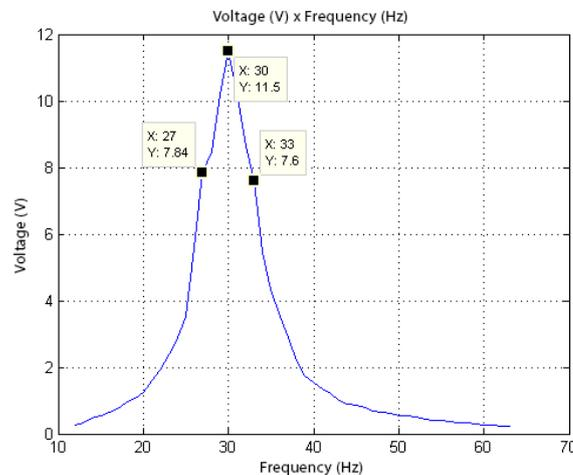
Figure 5. Voltage generated through frequency sweep
