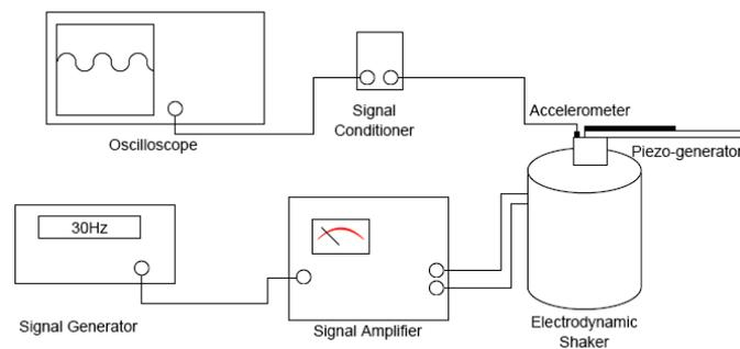
Figure 3. Schematic diagram for experimental validation of numerical model
