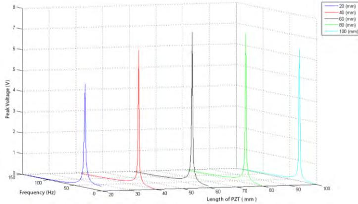
Figure 6. Peak voltages generated with different piezoelectric element length
