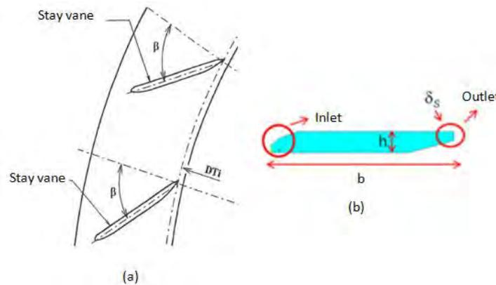
Figure 2. (a) Top view of a stay ring, with  $\beta = 55^\circ$  and  $DTi = 9.4$  m. (b) Stay vane cross section, with  $L = 2140$  mm,  $b = 755$  mm, and  $h = 90$  mm.
