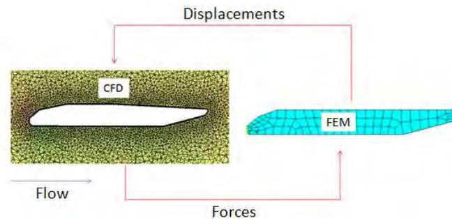
Figure 4. Interaction between two physics: structural and fluidic.
