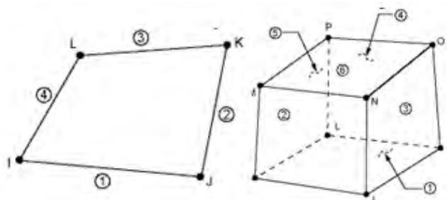
Figure 3: Finite elements utilized on structure and fluid mesh. 2D and 3D representation.
