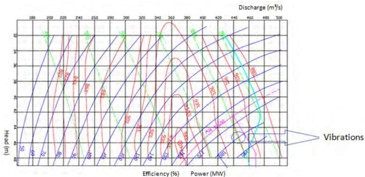
Figure 7. Hill chart for units from 05 to 20 at HPP Ilha Solteira. CESP,2012.
