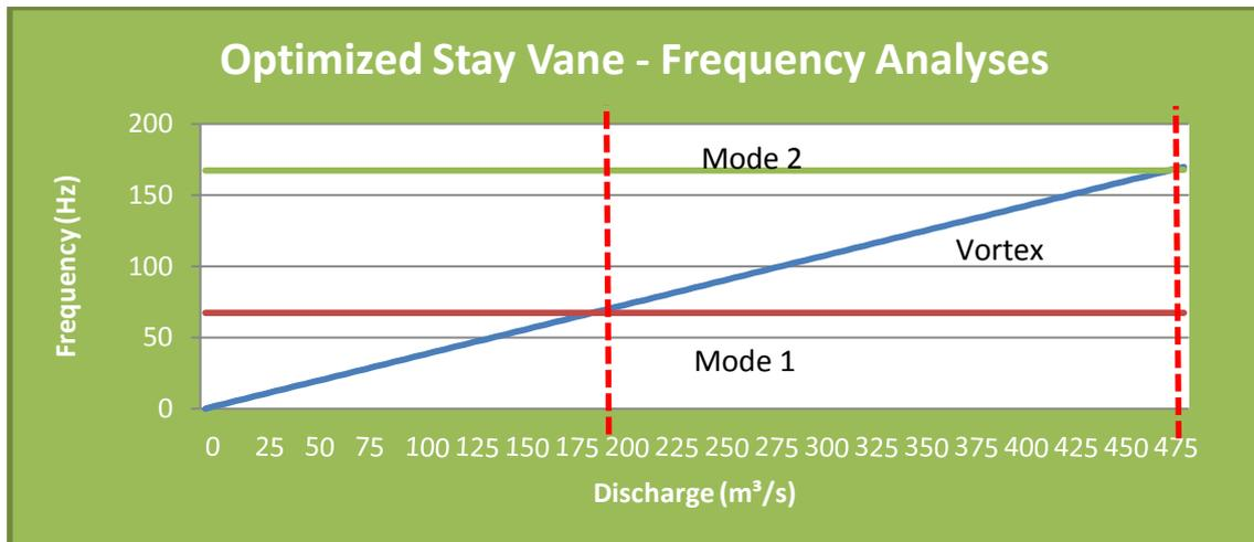
Figure 13. Frequency characteristics for optimized stay vane.
