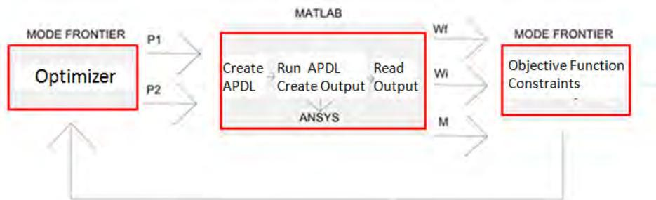
Figure 5. Computational optimization methodology flowchart.
