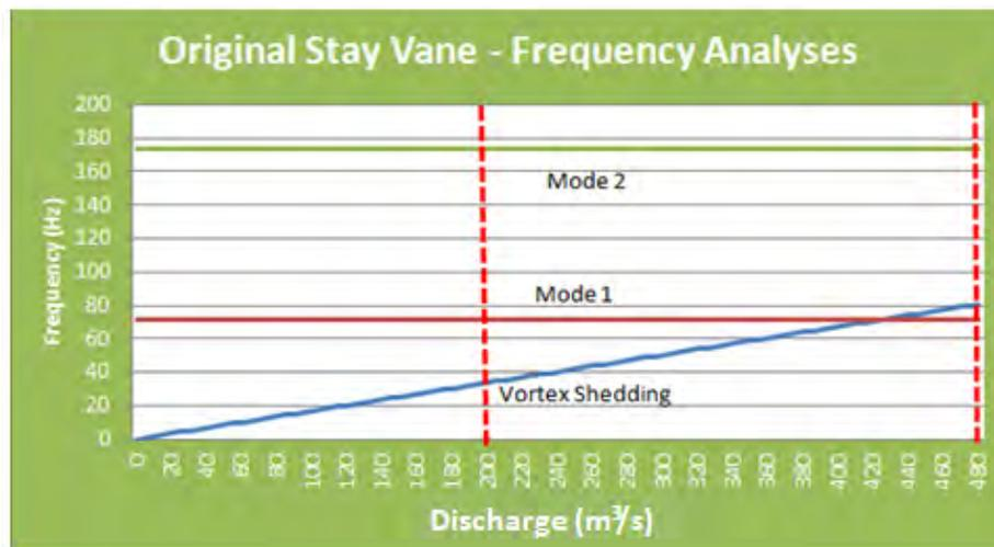
Figure 6. Shedding and natural frequencies for the original profile.
