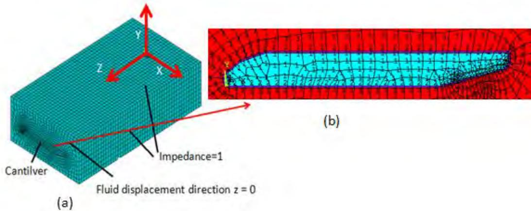
Figure 9. Boundary conditions and element types considered (“1” for structural and “2” and “3” for fluid).
