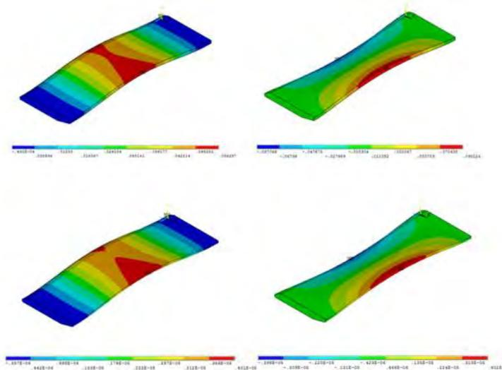
Figure 10. 1st and 2nd vibration modes in air (above) and water (below).
