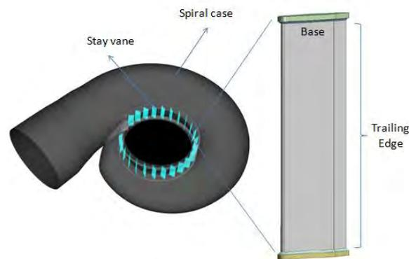
Figure 1. Spiral case and the set of stay vanes.
