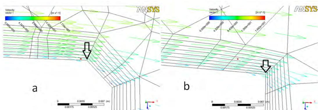
Figure 12. Separation of the flow around the stay vane. a) Original b) Optimized.
