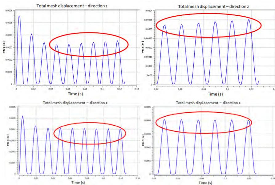
Figure 14. Maximum Total Mesh Displacement in Z direction (original structure above and optimized below). Highlighted in red from 0.04 s.
