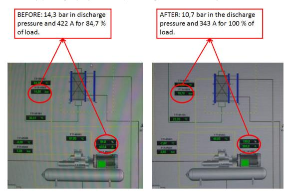
Figure 6. Measurement data of chiller 1 before and after the reform
