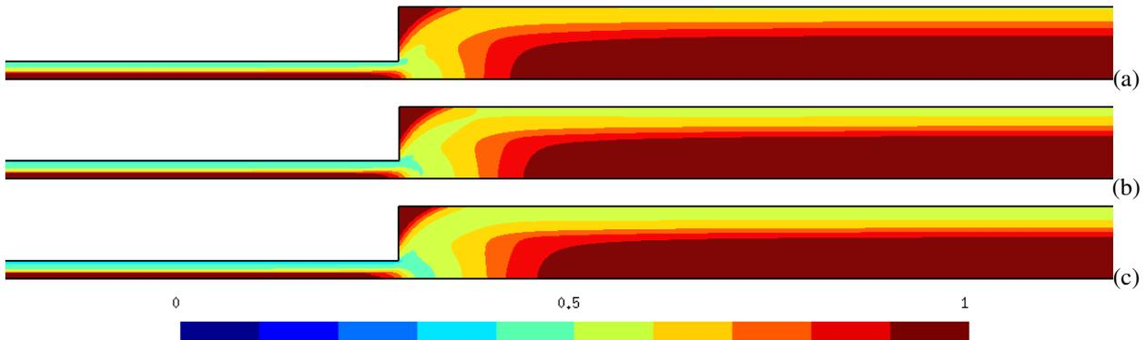
Figure 8. Structure Parameter field for  $\theta_0^* = 5$ ,  $t_{eq}^* = 1$ ,  $n = 0.5$  and: (a)  $J = 200$ : (b)  $J = 500$  and (c)  $J = 800$
