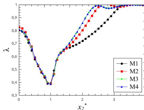
Figure 2. Structure Parameter profiles for  $\theta_0^* = 5$ ,  $J = 500$ ,  $n = 0.5$ ,  $t_{eq}^* = 1$  and  $x_1^* = 0$
