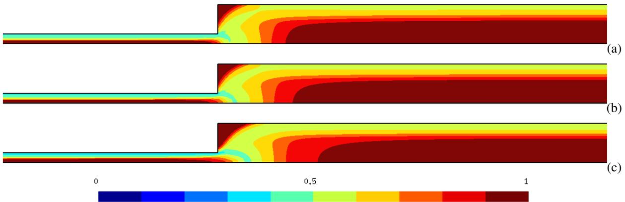
Figure 6. Structure Parameter field for  $t_{eq}^* = 1$ ,  $J = 500$ ,  $n = 0.5$  and: (a)  $\theta_0^* = 5$ ; (b)  $\theta_0^* = 25$  and (c)  $\theta_0^* = 100$
