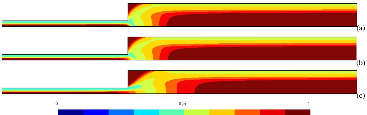
Figure 4. Structure Parameter field for  $\theta_0^* = 5$ ,  $J = 500$ ,  $n = 0.5$  and: (a)  $t_{eq}^* = 0.01$ ; (b)  $t_{eq}^* = 1$  and (c)  $t_{eq}^* = 10$
