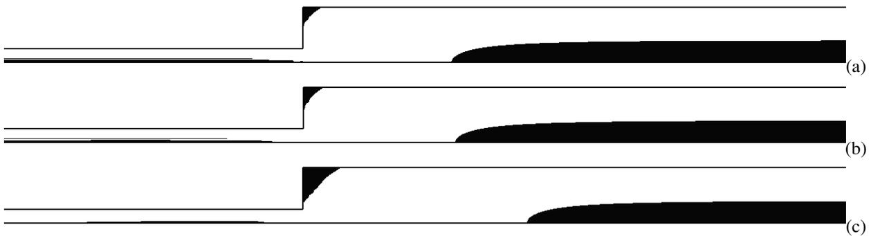
Figure 5. Unyielded Regions:  $\tau^*$ -isobands for  $\theta_0^* = 5$ ,  $J = 500$ ,  $n = 0.5$  and: (a)  $t_{eq}^* = 0.01$ ; (b)  $t_{eq}^* = 1$  and (c)  $t_{eq}^* = 10$
