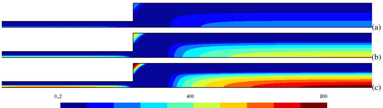
Figure 9. Structured Viscosity isobands for  $\theta_0^* = 5$ ,  $t_{eq}^* = 1$ ,  $n = 0.5$  and: (a)  $J = 200$ : (b)  $J = 500$  and (c)  $J = 800$
