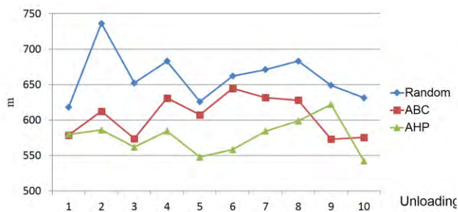
Figure 4. Comparison among random, ABC and AHP allocations for cost (distance traveled) and time spent.
