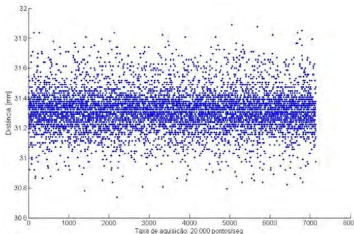
Figure 1. Example point cloud acquired by laser sensor for a fixed distance
