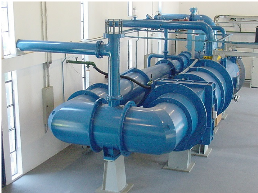
Figure 2. View of the aerodynamic circuit of TTP 17 meters long
